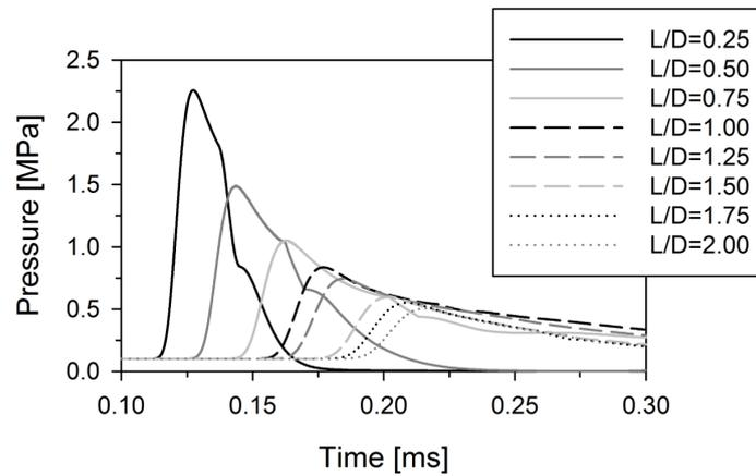
*Fig. 8. Pressure values at the distance of 35 cm from the centre of the TNT charge*
