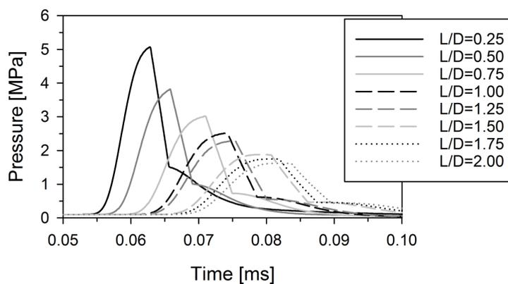
Fig. 7. Pressure values at the distance of 20 cm from the centre of the TNT charge
