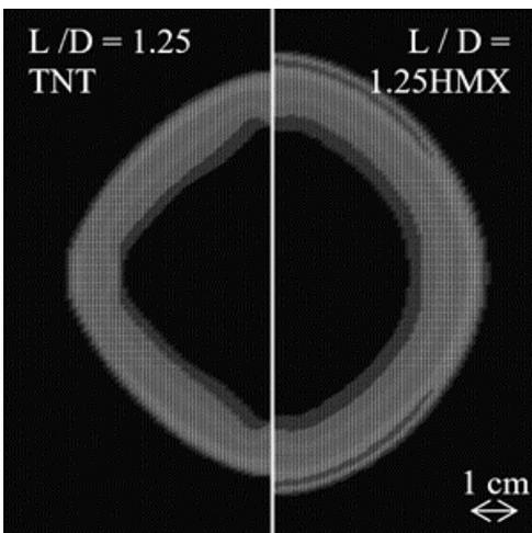
Fig. 5. Shape of the blast wave 0.2 ms after initiating the detonation for charge with L/D ratio of 1.25
