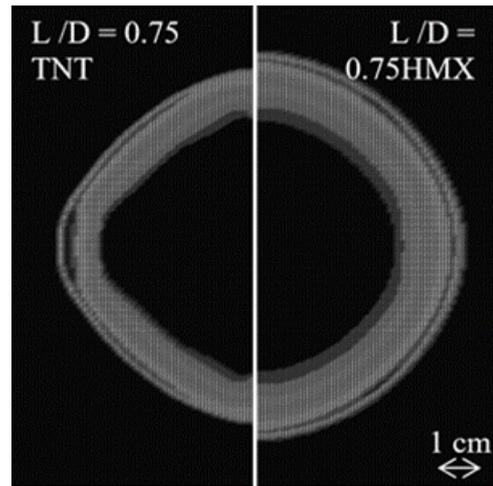
Fig. 4. Shape of the blast wave 0.2 ms after initiating the detonation for charge with L/D ratio of 0.75
