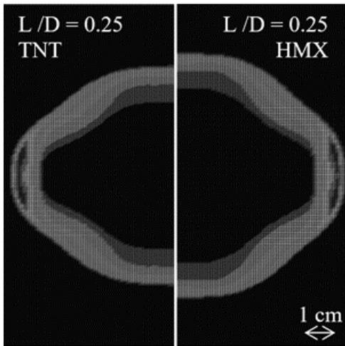
Fig. 3. Shape of the blast wave 0.2 ms after initiating the detonation for charge with L/D ratio of 0.25
