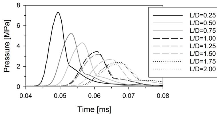
*Fig. 9. Pressure values at the distance of 20 cm from the centre of the HMX charge*
