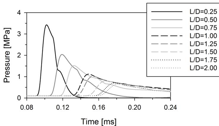
*Fig. 10. Pressure values at the distance of 35 cm from the centre of the HMX charge*
