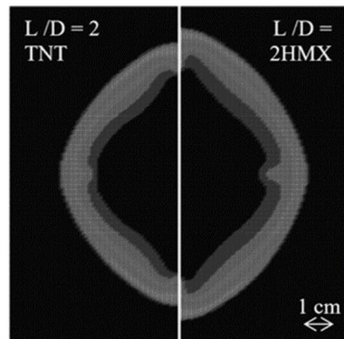
Fig. 6. Shape of the blast wave 0.2 ms after initiating the detonation for charge with L/D ratio of 2
