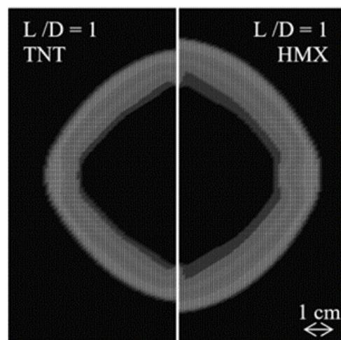
Fig. 2. Shape of the blast wave 0.2 ms after initiating the detonation for charge with  $L/D$  ratio of 1
