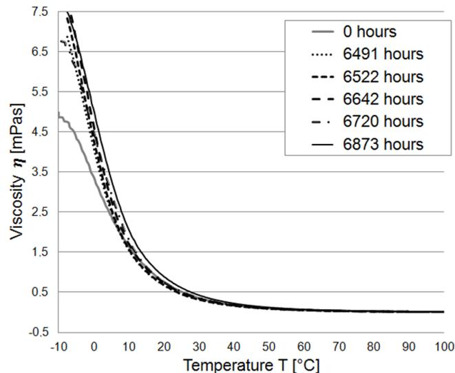
Fig. 2. Graph of viscosity-temperature changes for Marinol RG 1240 after different time of usage
