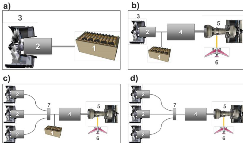
Fig. 2. Comparison of different types of architectures: a) full-electric propulsion system, b) parallel hybrid propulsion system, c) series hybrid, d) turboelectric. 1 – battery, 2 – electric motor, 3 – fan or propeller, 4 – generator, 5 – turbine engine, 6 – fuel tanks, 7 – power buss
