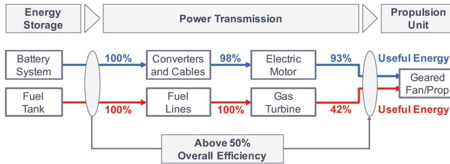
Fig. 3. Comparison of energy conversion efficiency for the electric propulsion system and for the standard propulsion system with internal combustion engine [6]
