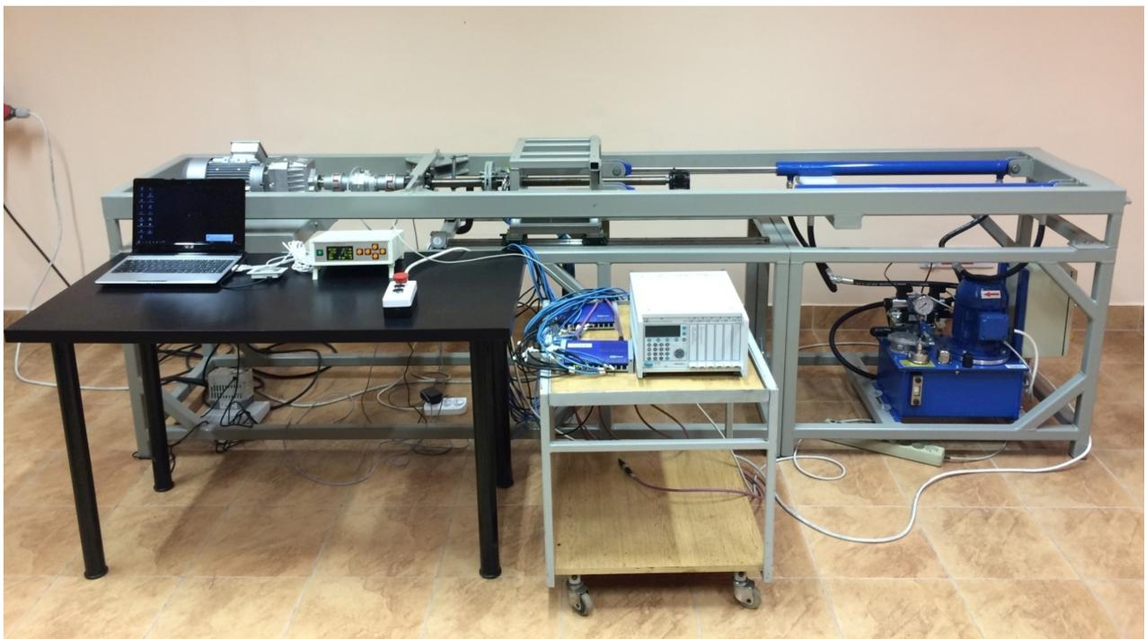
*Fig. 2. A test stand for lead screws*
