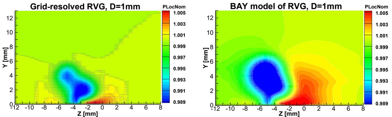
Fig. 7. Normalised local total pressure contour at  $X = 4.6$  cm behind grid-resolved RVG in the left plot and its BAY model in the right plot, diameter  $D = 1$  mm
