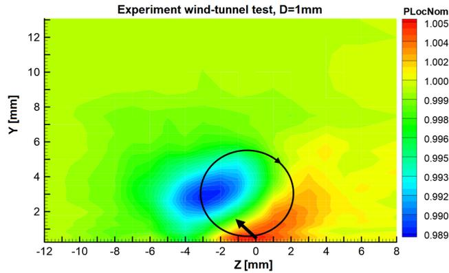
Fig. 6. Normalized local total pressure contour at  $X = 4.6$  cm behind RVG measured in wind-tunnel experiment, diameter  $D = 1$  mm [8]
