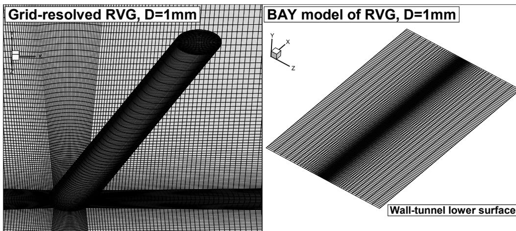
Fig. 3. Comparison of used meshes for computations – the mesh, which resolve the shape of RVG (left figure) and mesh on lower wall-tunnel surface for which the BAY model was used (right figure)
