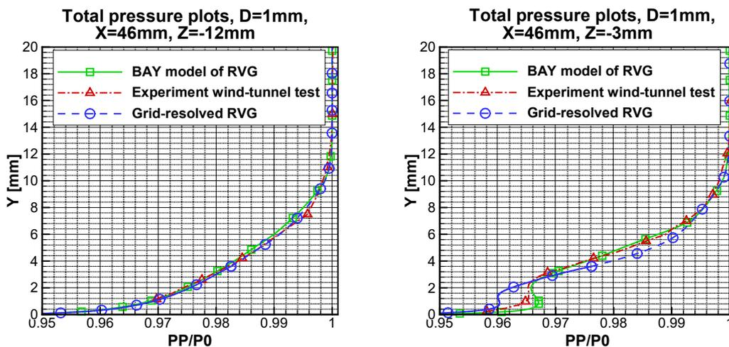
Fig. 8. Plots of total pressure profile in boundary layer in  $X = 46$  mm behind RVG of diameter  $D = 1$  mm for experiment wind-tunnel result, grid-resolved RVG and its BAY model
