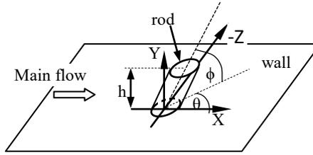
Fig. 1. Schematic of RVG orientation in computational domain [8] (left plot) and
