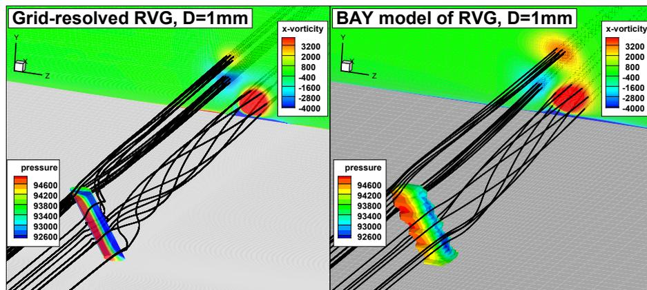
Fig. 5. Contour of  $x$ -vorticity at slice 4 cm behind RVG with pathlines and static pressure contour on RVG surface (left plot) and on the surfaces of cells, where source term is added in BAY model (right plot)
