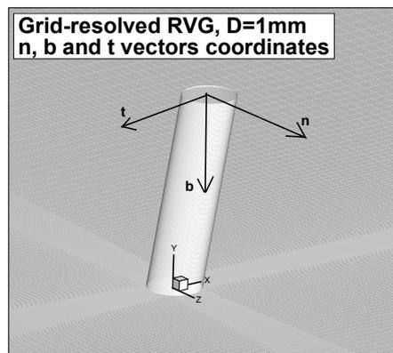
Fig. 2. Spatial orientation of BAY model vectors referenced to rod coordinates
