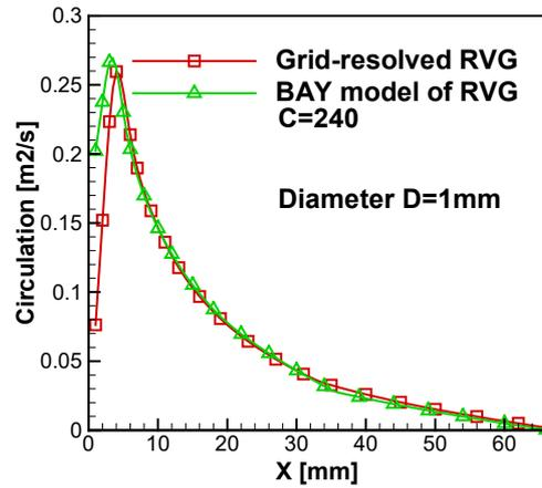
Fig. 4. Plot of circulation behind rod vortex generator placed in  $X = 0$  m
