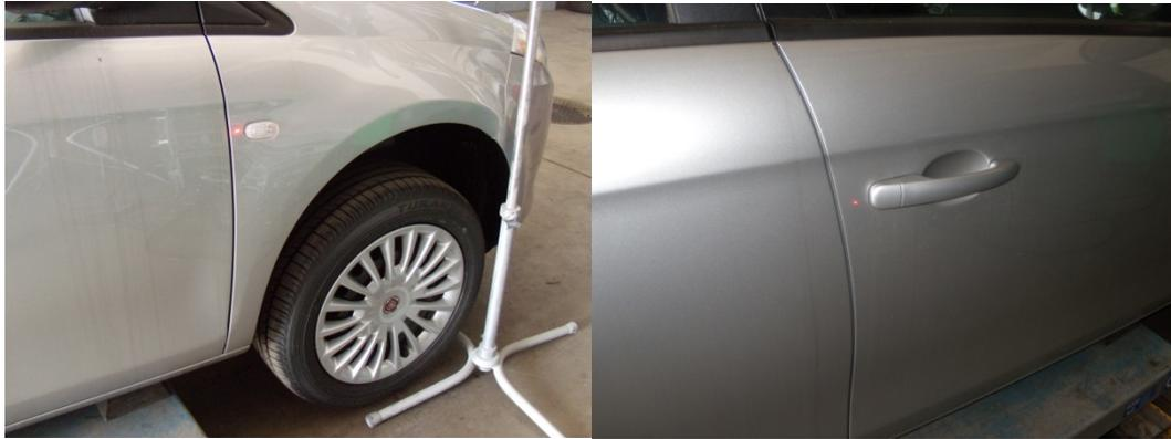
Fig. 1. LDV targets on the wheel arch (left side) and passenger's door
