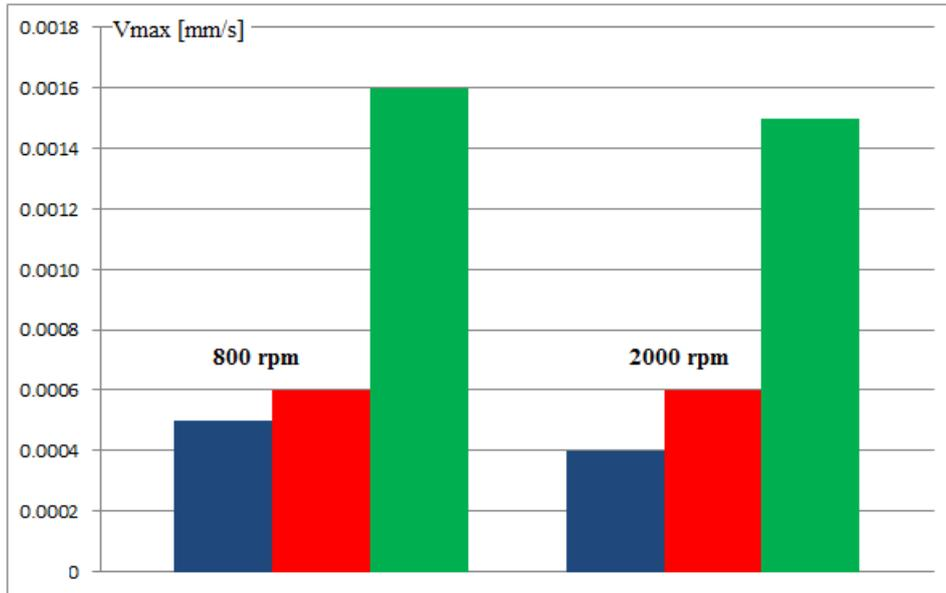
Fig. 9. Comparison of maximum relative vibration velocity measured on the passenger's door for a car model equipped with 3 different engines; blue – 1.4 L spark ignition engine (90 KM), red – supercharged spark ignition engine (120 KM), green – 1.6 L compression ignition engine (105 KM)
