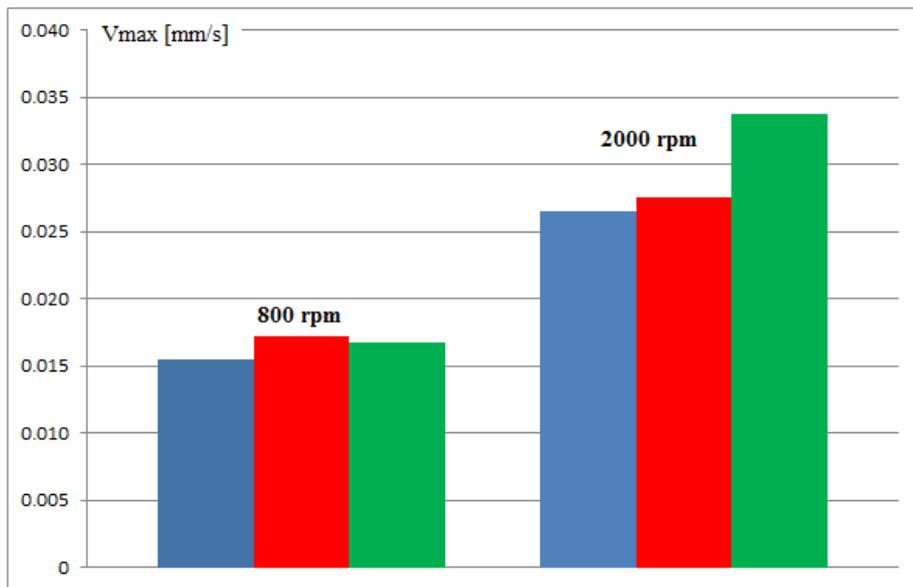
Fig. 7. Comparison of maximum relative vibration velocity measured on the engine mount bracket for a car model equipped with 3 different engines; blue – 1.4 L spark ignition engine (90 KM), red – supercharged spark ignition engine (120 KM), green – 1.6 L compression ignition engine (105 KM)
