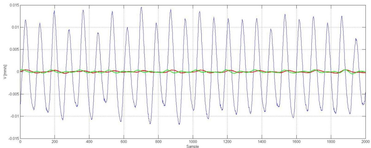
Fig. 2. Absolute vibration velocity levels for a vehicle with 1.4 L spark ignition engine (90 KM), idle speed (800 rpm); blue – on the engine mount bracket, red – on the wheel arch, green – on the passenger's door
