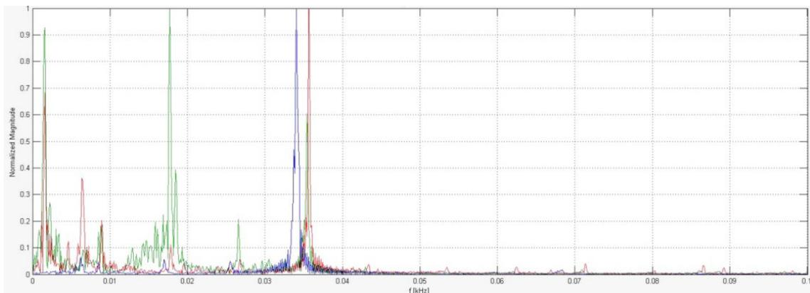
Fig. 4. Relative vibration velocity levels (frequency response) for a vehicle with 1.4 L spark ignition engine (90 KM), idle speed (2000 rpm); blue – on the engine mount bracket, red – on the wheel arch, green – on the passenger's door
