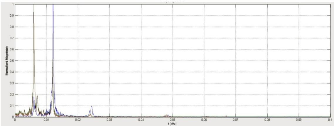
Fig. 3. Relative vibration velocity levels (frequency response) for a vehicle with 1.4 L spark ignition engine (90 KM), idle speed (800 rpm); blue – on the engine mount bracket, red – on the wheel arch, green – on the passenger's door
