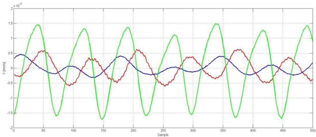
Fig. 5. Discrete relative vibration levels for three vehicles: blue – non-supercharged 1.4 L spark ignition engine, red – 1.4 L supercharged engine, green – 1.6 L compression ignition engine; the measurement taken on the passenger's door, idle speed 800 rpm
