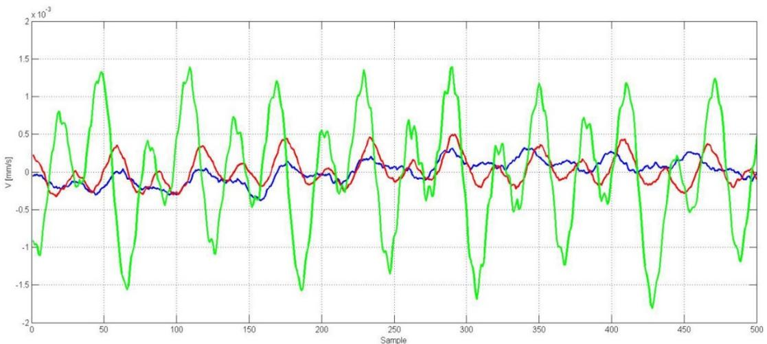
Fig. 6. Discrete relative vibration levels for three vehicles: blue – non-supercharged 1.4 L spark ignition engine, red – supercharged 1.4 L engine, green – 1.6 L compression ignition engine; the measurement taken on the passenger's door, idle speed 2000 rpm
