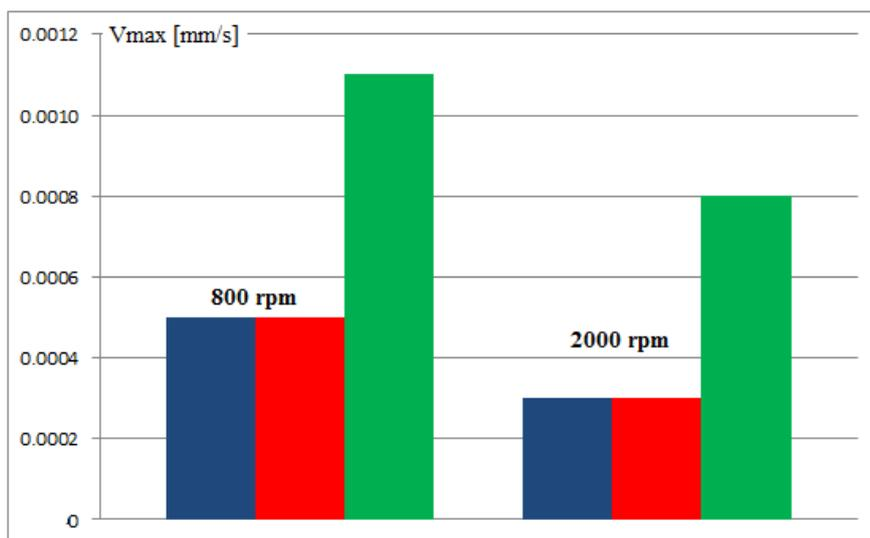
Fig. 8. Comparison of maximum relative vibration velocity measured on the wheel arch body for a car model equipped with 3 different engines; blue – 1.4 L spark ignition engine (90 KM), red – supercharged spark ignition engine (120 KM), green – 1.6 L compression ignition engine (105 KM)
