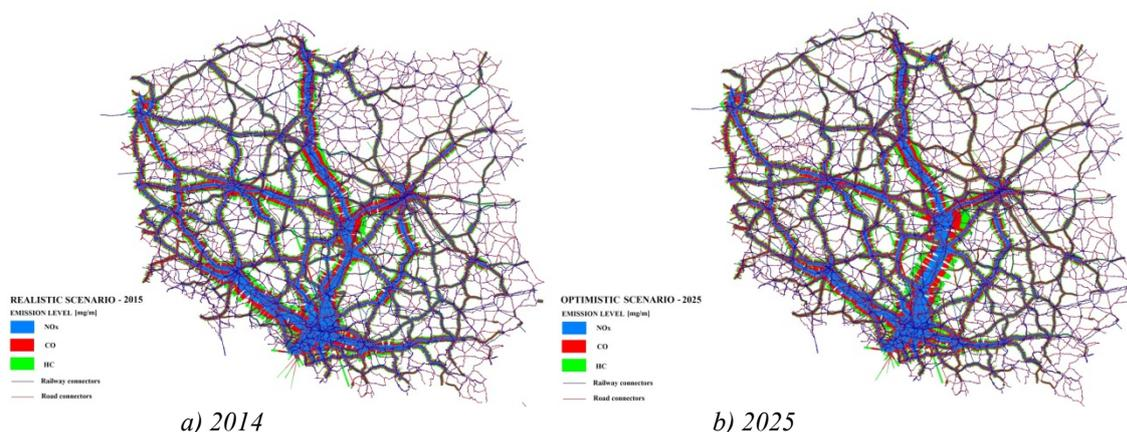
Fig. 7. Exhaust emission of harmful compounds due to the EURO standards a) in 2014 – for the current vehicles structure, b) in 2025 for the change in vehicle structure
