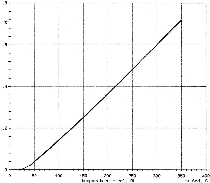
Fig. 8. Course of the relative piston elongation  $\Delta L/L_0$  versus temperature during heating and cooling for the composite alloy
