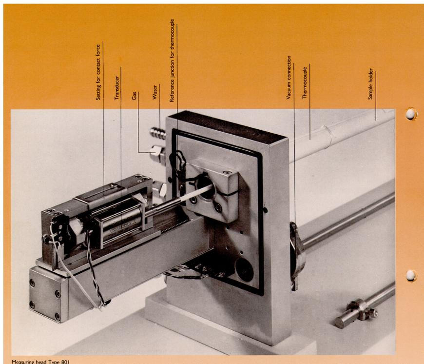
Fig. 4. View of the measuring-head of the extension
