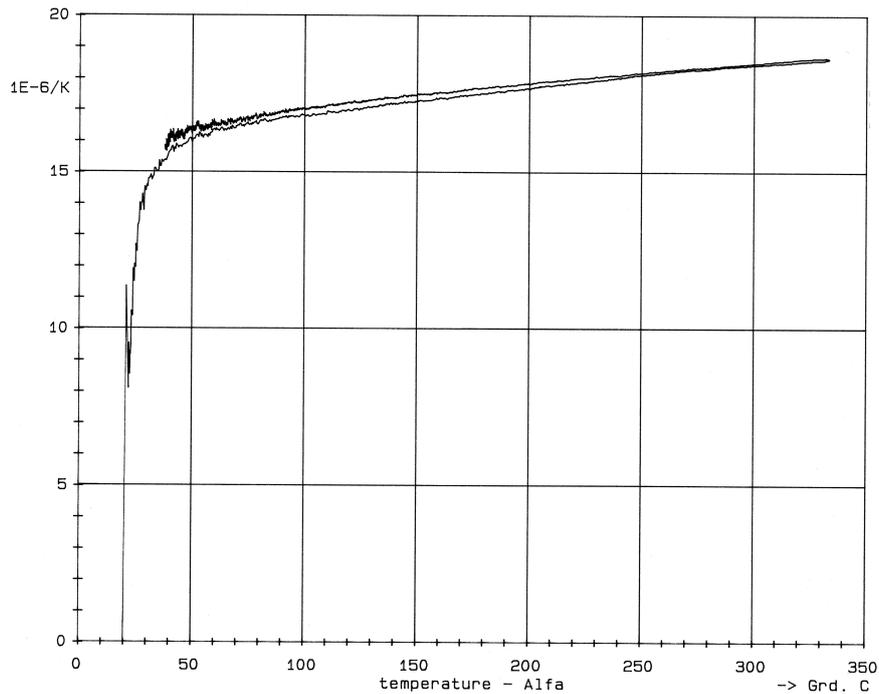
Fig. 6. Course of coefficient of linear thermal expansion  $\alpha$  versus temperature during heating and cooling for composite alloy
