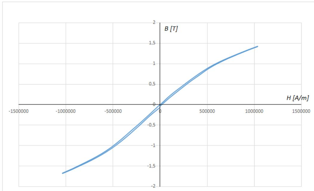
Fig. 7. B-H curve for sample having a thickness 0.9 mm
