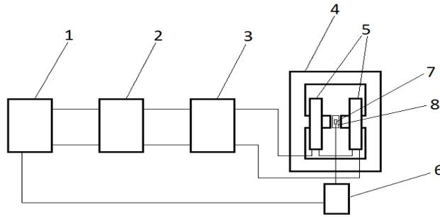
Fig. 2. Test stand scheme: 1 – PC with data control -measurement application, 2 – power supply, 3 – electromagnetic relay, 4 – yoke, 5 – coils, 6 –gaussmeter , 7 – measuring probe, 8 – measuring gap
