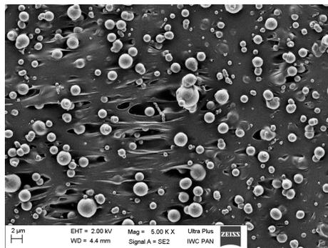
Fig. 1. SEM microstructure of MR composite revealed on a surface of sample containing CIP HS
