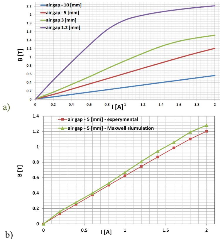
Fig. 4. The electromagnet calibration: a) experimental for different air gap; b) compare with Maxwell simulation
