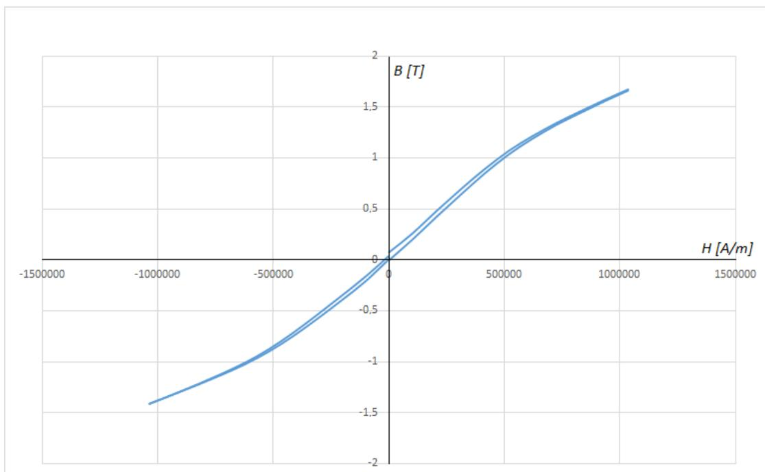
Fig. 6. B-H curve for sample having a thickness 0.8 mm
