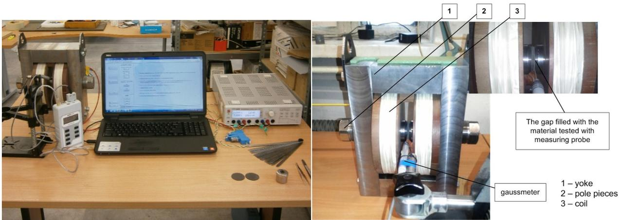
Fig. 5. Magnetic induction measurement on the working station with the magnetorheological elastomer
