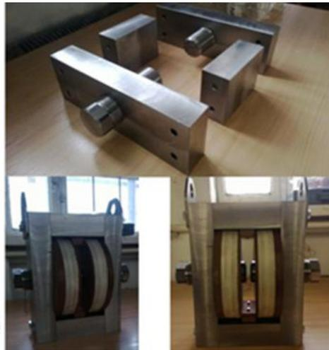
Fig. 3. Electromagnet yoke
