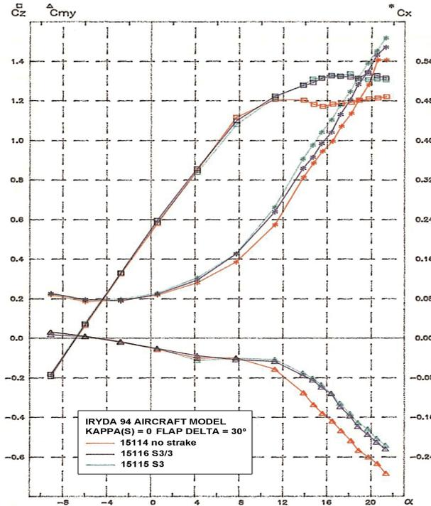
Fig. 2. Aerodynamic characteristics of aircraft model  $C_z(\alpha)$ ,  $C_x(\alpha)$  and  $C_{my}(\alpha)$  with and without strake in various variants (slotted flap  $\delta_\kappa = 30^\circ$ ) [6]
