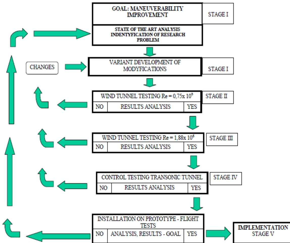
Fig. 1. Design and testing method algorithm [3]
