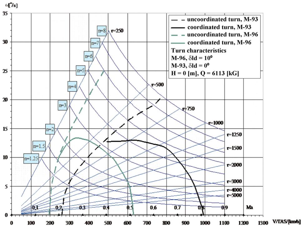
Fig. 8. Characteristics of steady and unsteady turn radius versus speed for I-22 "Iryda" plane before and after its modernization with the flap in a manoeuvring position for height  $H = 0$  m [4, 10]
