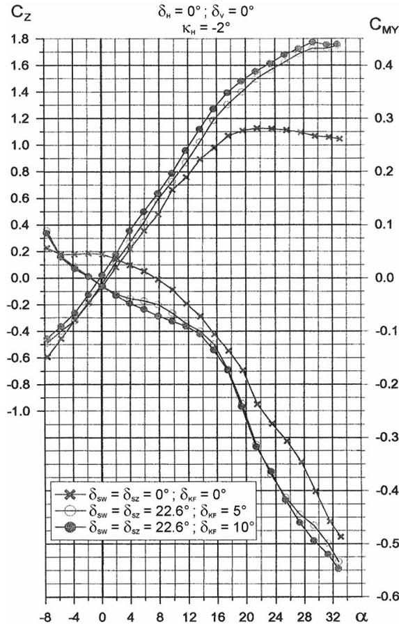
Fig. 4. Aerodynamic characteristics of the aircraft model  $C_x(\alpha)$ ,  $C_z(\alpha)$  and  $C_{My}(\alpha)$  with the selected variant of strake with Fowler flap and hidden slot as well flap and slot in a manoeuvring position angled by  $\delta_{KF} = 5^\circ$  and  $\delta_{KF} = 10^\circ$  [7]
