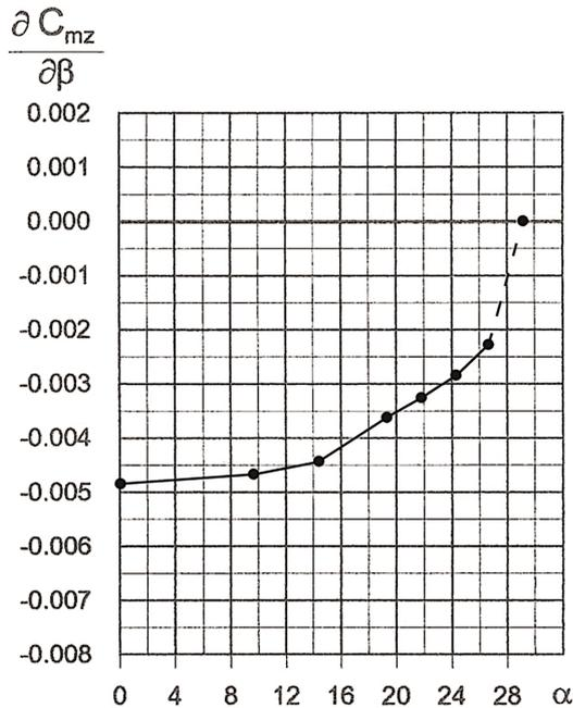
Fig. 5. Dependence of  $\partial C_{mz} / \partial \beta$  on the wing angle of attack for the tested configurations of the model of aircraft with a band and a swivelled wing flap in the manoeuvring position [7]
