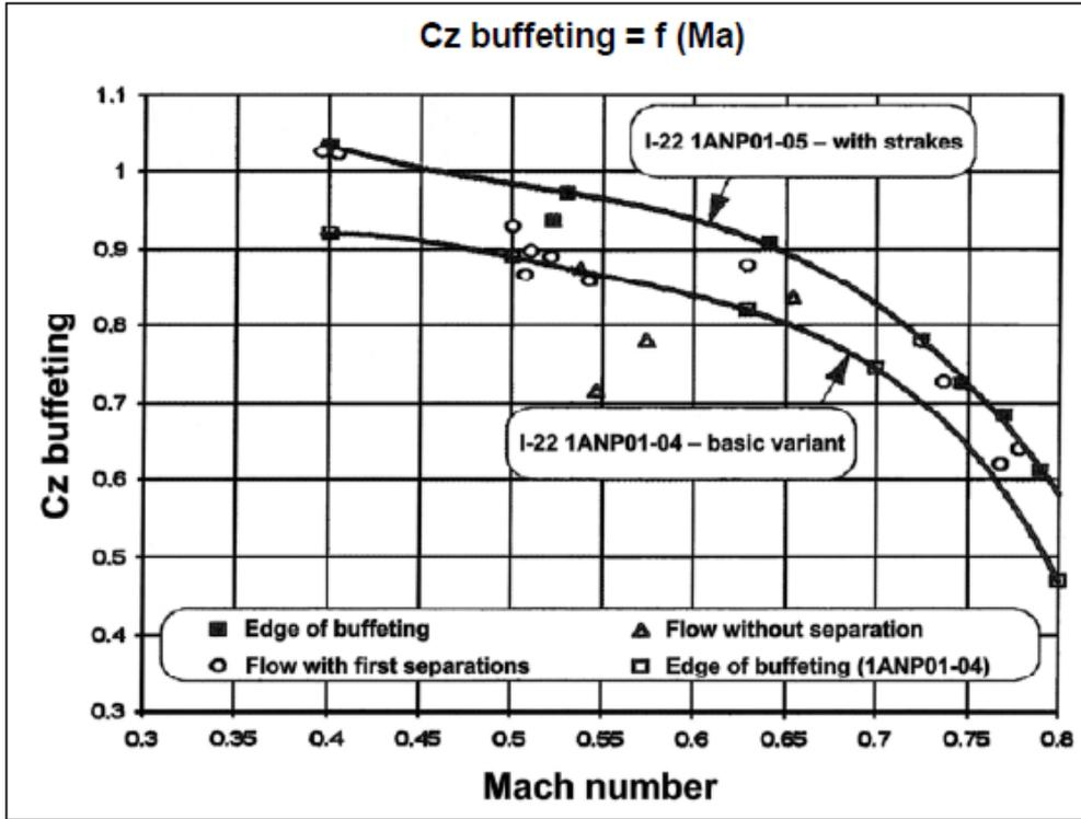
Fig. 7. Comparison of the lift factor at initial buffeting vibrations of aircraft prototype with mounted strake and without mounted strake [5, 12]
