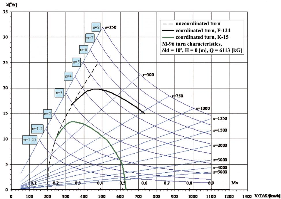
Fig. 9. Characteristics of steady and unsteady turn for aircraft with mounted LERX and the flap in a manoeuvring position with thrust;  $2 \times 1500$  daN and thrust  $2 \times 2833$  daN for height;  $H = 0$  m [4, 10]
