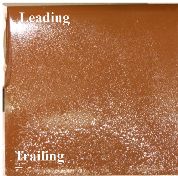
Fig. 9. Oil flow visualization for  $Ma=0.2$ ,  $\alpha=12^\circ$
