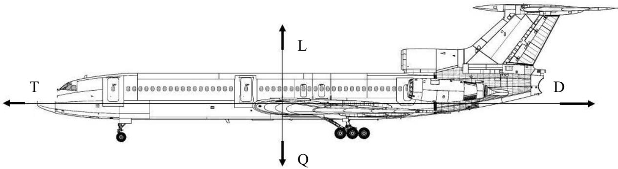
Fig. 1. The distribution of forces on the example of the aircraft
