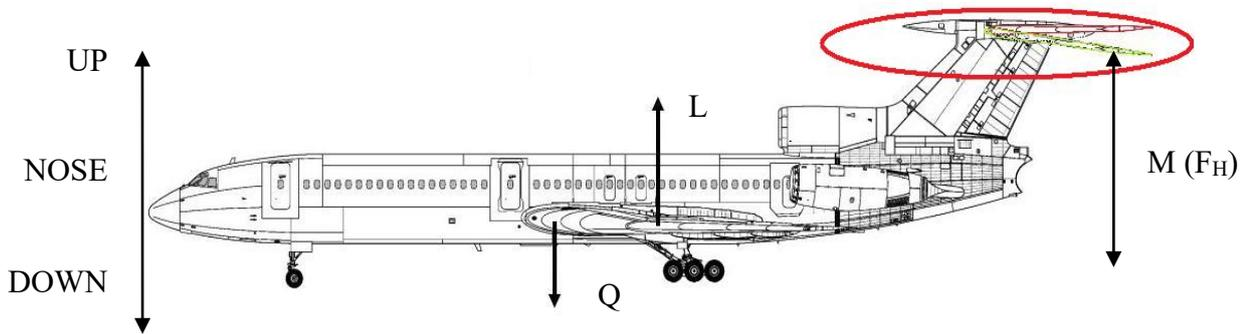
Fig. 3. The principle of operation of the horizontal tail of the aircraft
