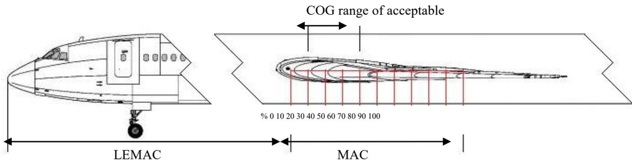
Fig. 5. Graphical representation of the allowable position COG
