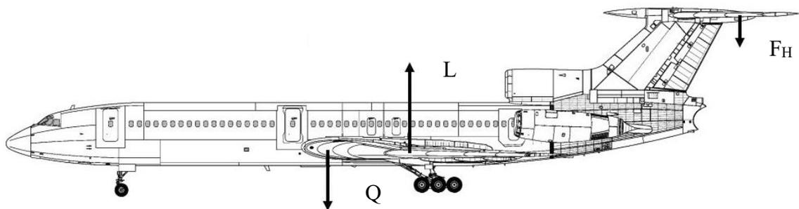
Fig. 2. The distribution of forces on the example of the aircraft
