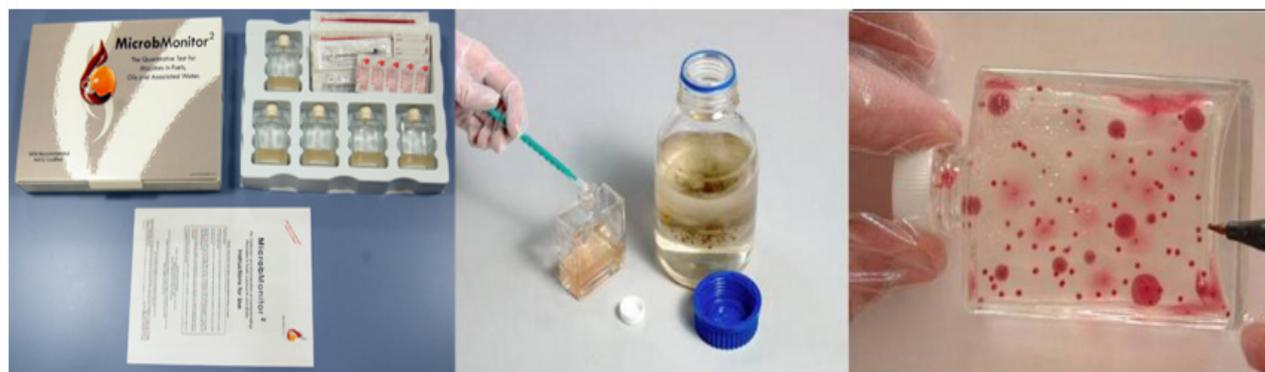
*Fig. 4. Detection of microorganisms using a special kit MicrobMonitor [12]*
