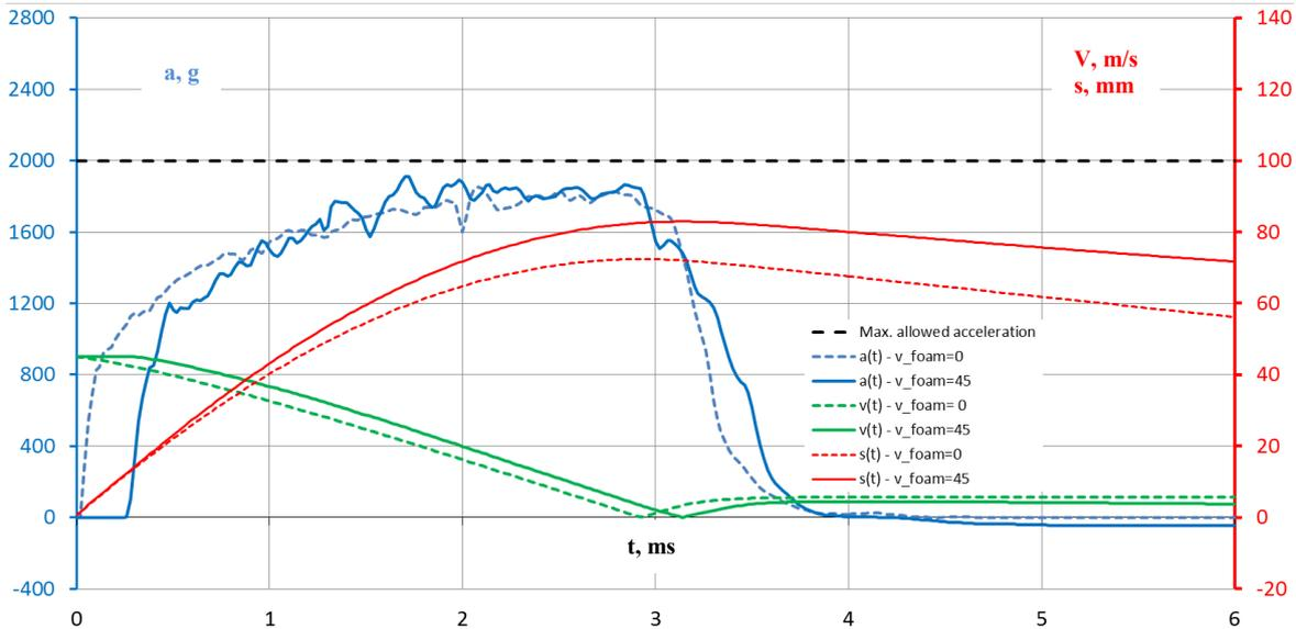
Fig. 9. The results for real energy absorption module FEM simulation – Puren 145 material
