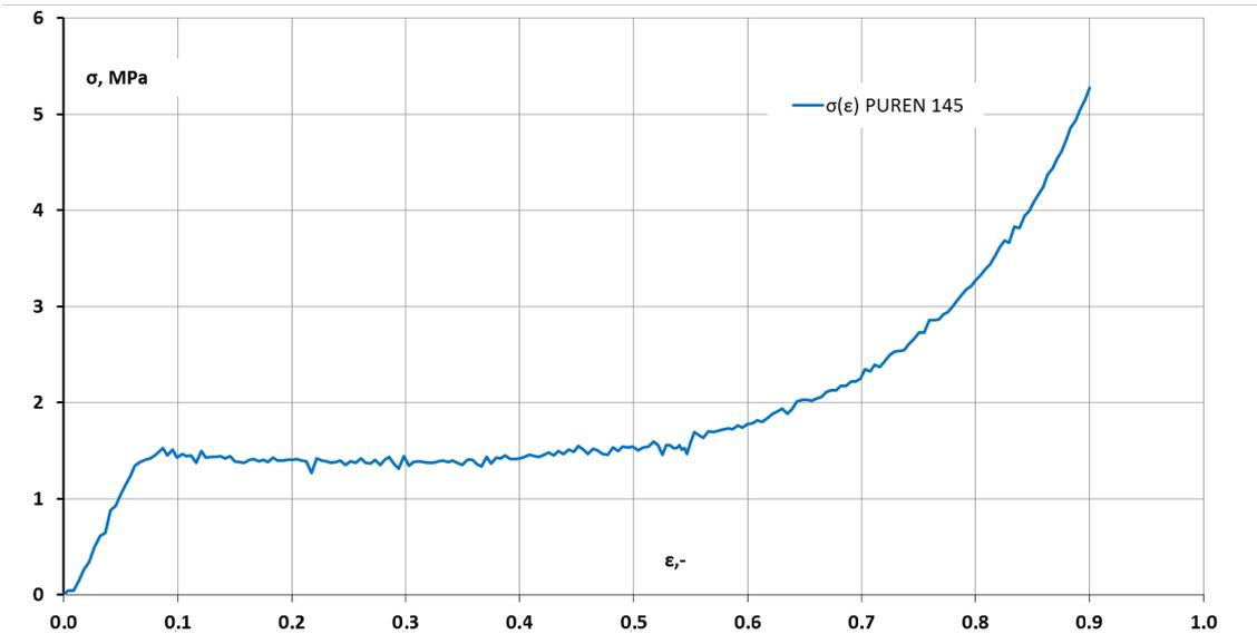
*Fig. 4. Stress versus strain curve for Puren145 material used in FE model*
