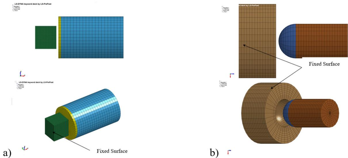
*Fig. 5. Finite element models representing tests of a) cube-shaped samples b) full-scale object*
