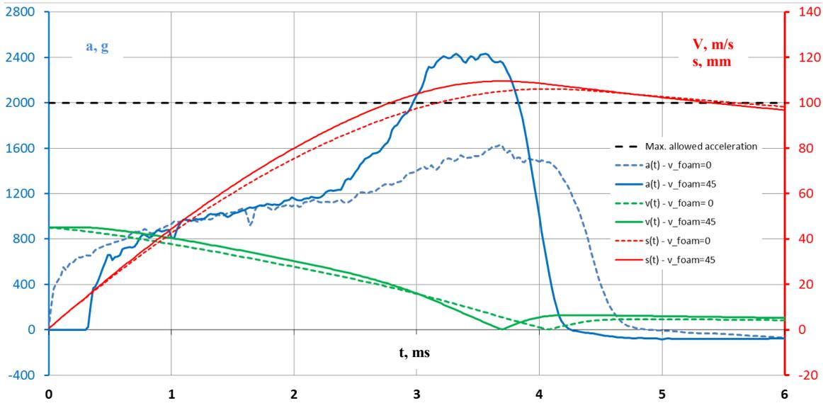
Fig. 8. The results of real shaped object FEM simulation – Puren 100 material
