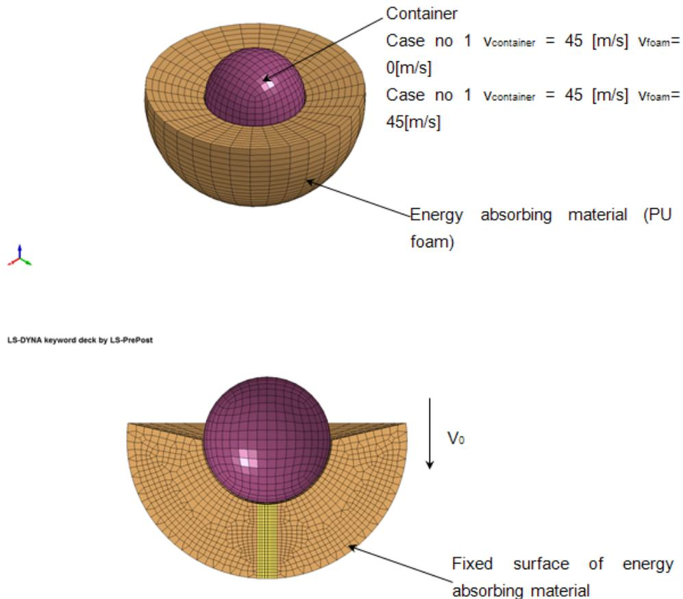
Fig. 7. Finite FEM model of container surrounded by energy absorbing material with initial and boundary conditions shown
