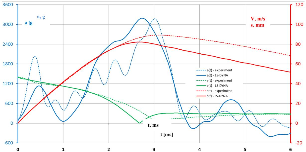
Fig. 6. Finite Comparison of simulation and laboratory test results for Puren145 material
