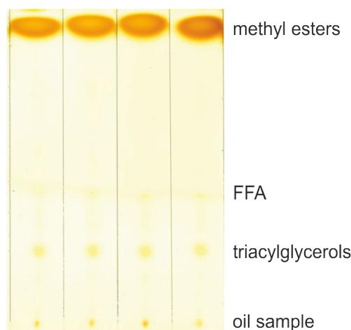
Fig. 1. TLC chromatograms of esters obtained by single-base esterification from different oils: a) reference sample, b) 15 min ultrasounds treatment, c) 30 min ultrasounds treatment, d) 60 min ultrasounds treatment
