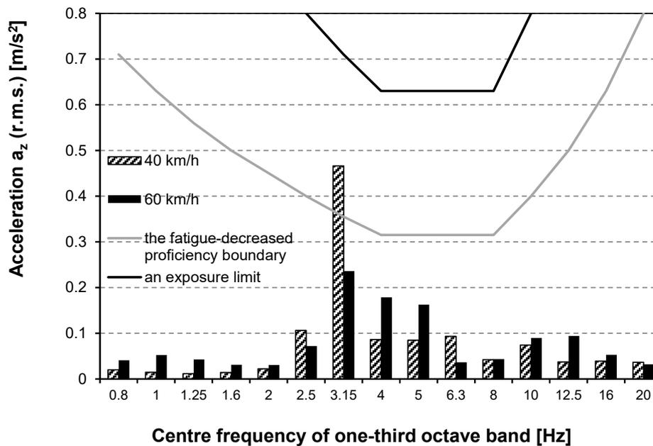
Fig. 6. RMS of vertical acceleration on seat no. 1 – asphalt road,  $v = 40$  and  $60 \text{ km/h}$
