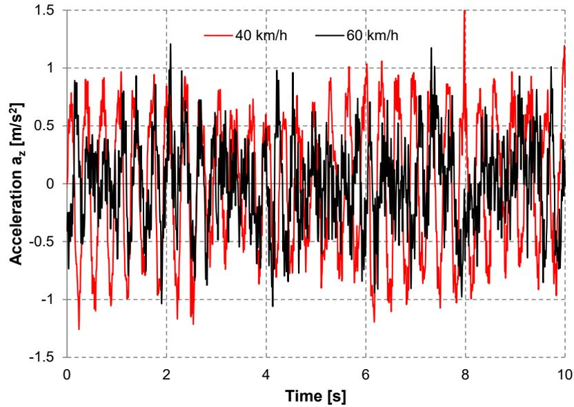
Fig. 4. Vertical accelerations on seat no. 1 – asphalt road,  $v = 40$  and  $60$  km/h
