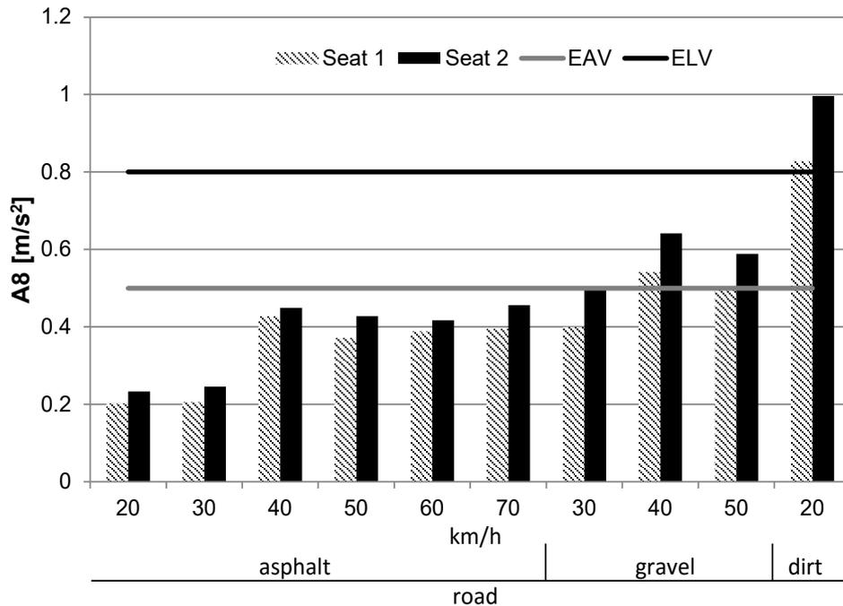
Fig. 7. The levels of daily exposure values to whole body vibrations on seat no. 1 and 2 – asphalt road,  $v = 40$  and  $60$  km/h
