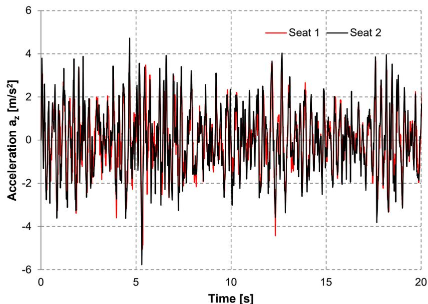
Fig. 3. Vertical accelerations on seats – dirt road,  $v = 20$  km/h
