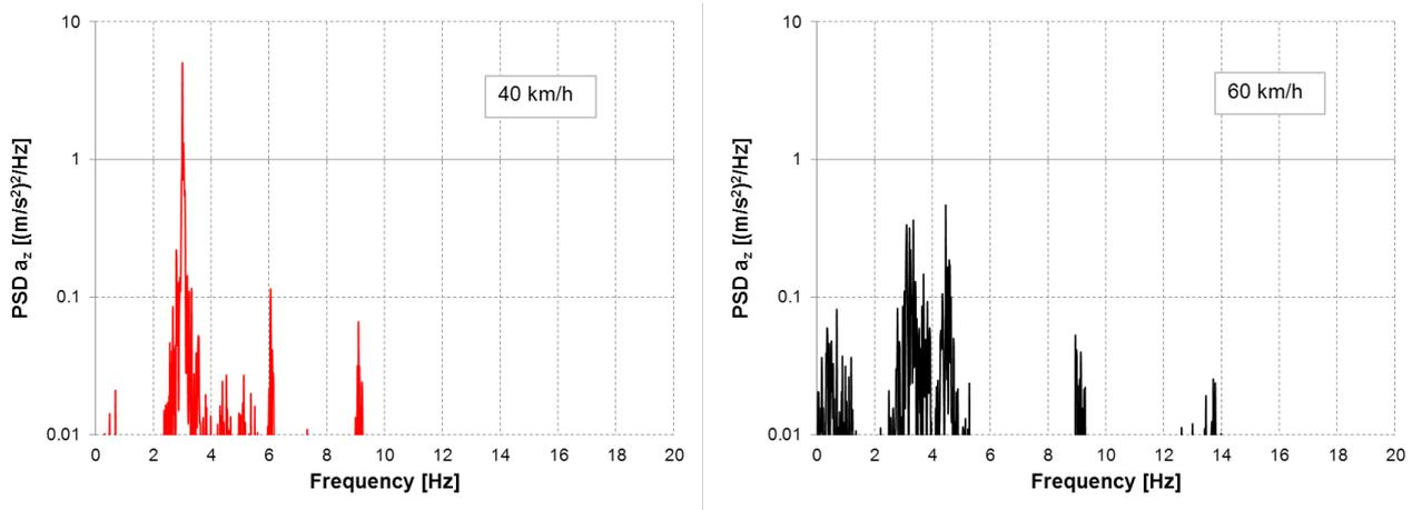
Fig. 5. Power spectra density of the accelerations on seat no. 1 – asphalt road,  $v = 40$  and  $60$  km/h
