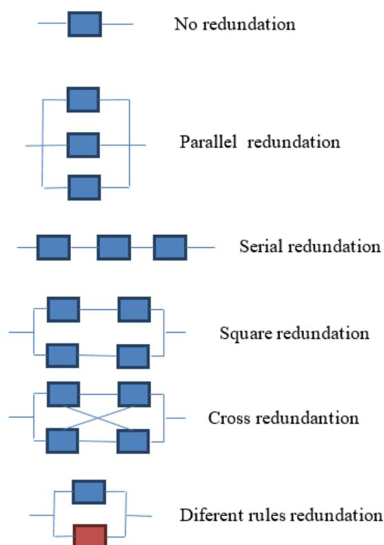
Fig. 4. The redundant systems
