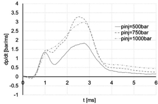
Fig. 11. ROPR ( $dp/dt$ ) for various injection pressure (fuel glycerol, 70/590)
