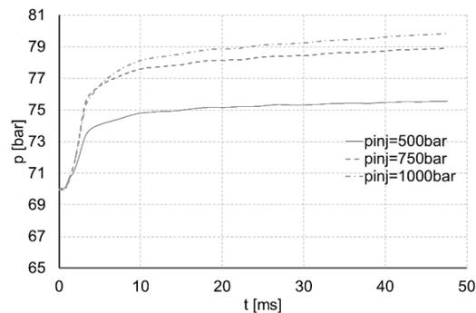
Fig. 9. Combustion pressure increase for various injection pressure (fuel glycerol, 70/590)
