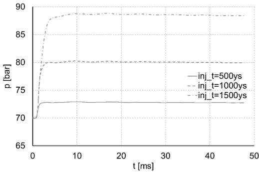
Fig. 12. Combustion pressure increase for various injection duration (fuel LFO, 70/590)
