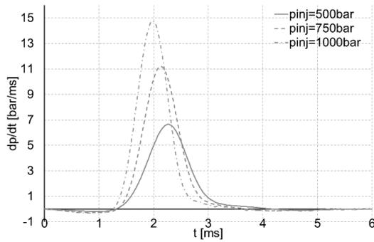
Fig. 6. ROPR ( $dp/dt$ ) for various injection pressure (fuel LFO, 55/550)
