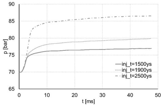
Fig. 13. Combustion pressure increase for various injection duration (fuel glycerol, 70/590)
