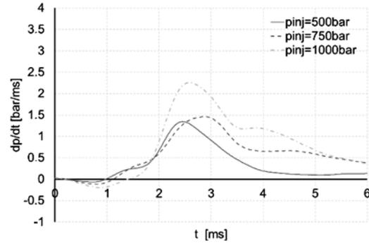
Fig. 7. ROPR ( $dp/dt$ ) for various injection pressure (fuel glycerol, 55/550)
