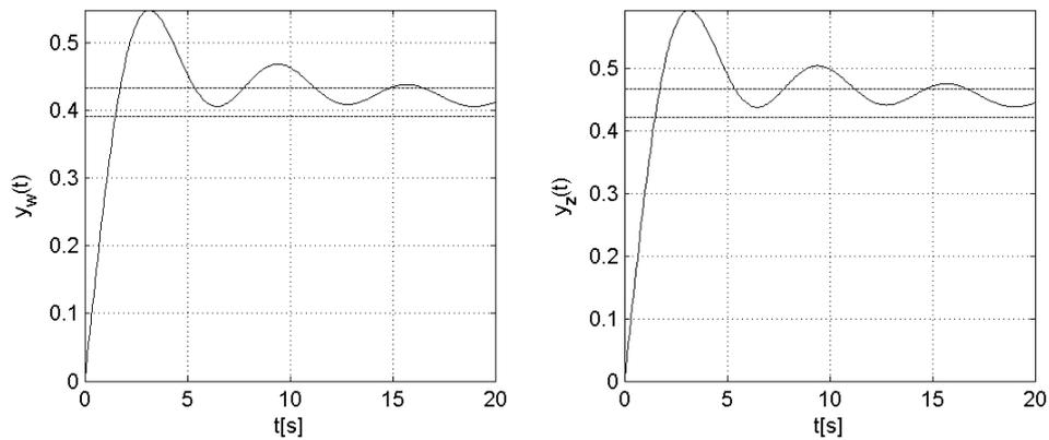
Fig. 6. Step responses of the engine on ground  $y_w(t)$  and in-flight  $y_z(t)$  for steady state of the engine work.
