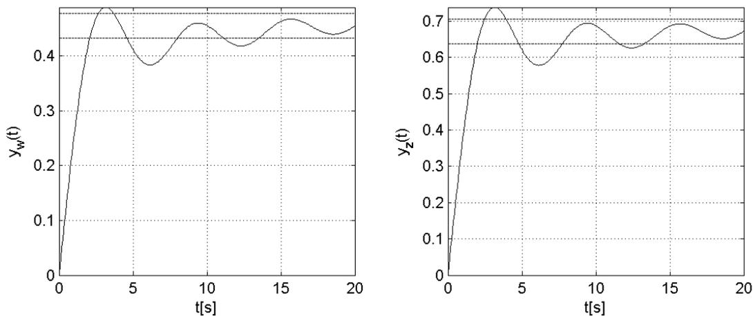
Fig. 5. Step responses of the engine on ground  $y_w(t)$  and in-flight  $y_z(t)$  for sudden deceleration of the engine
