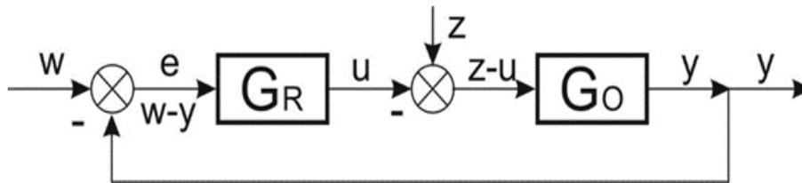
Fig. 1. Scheme of the simplified aircraft engines automatic control system, where:  $G_R$  – controller transfer function,  $G_O$  – object transfer function,  $w$  – input signal delivered by the engine control lever,  $z$  – input signal (disturbances),  $y$  – output signal (engine rotational speed),  $e = w - y$  – input signal for the controller,  $u$  – output signal from the controller [4, 6, 7]
