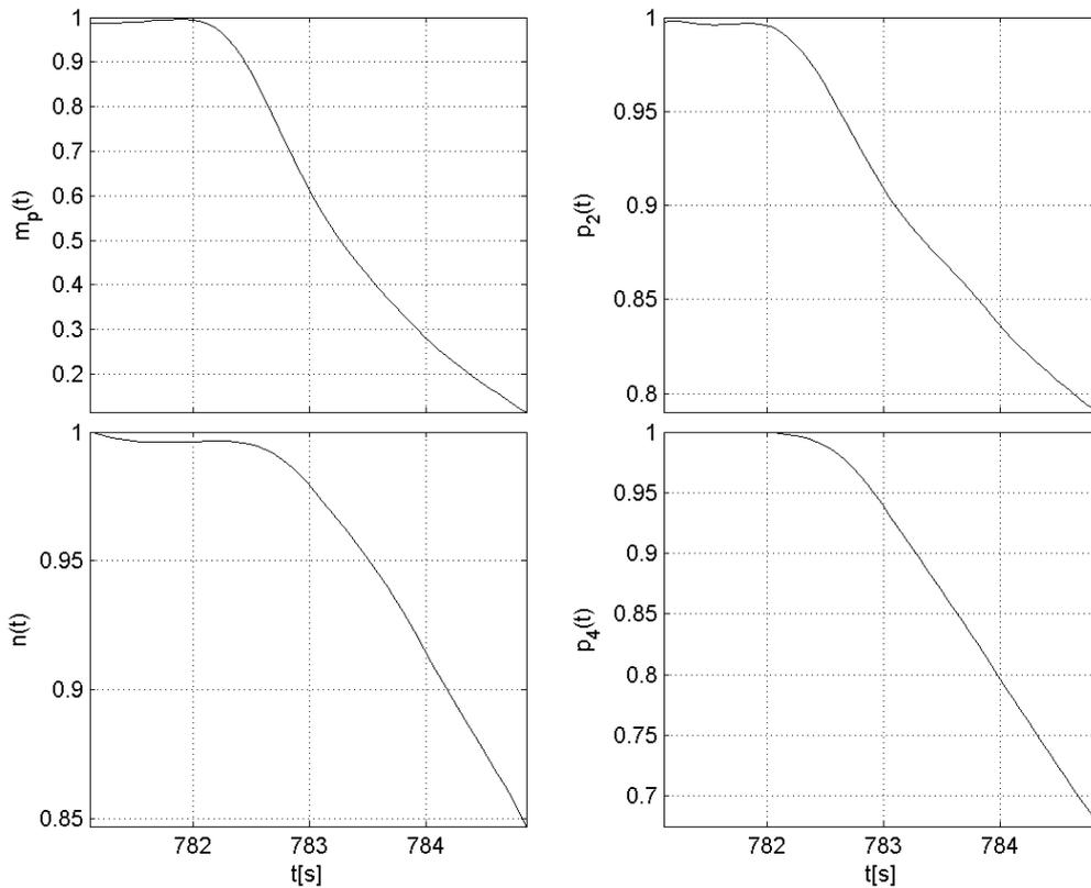
Fig. 3. The plots of standardized signals registered during sudden deceleration
