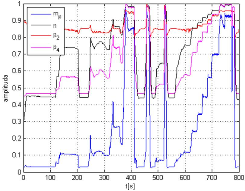
Fig. 2. The plots of standardized signals registered during K15 engine ground tests., where  $p_2$  – input signal, air pressure downstream of the compressor and  $m_p$  – input signal, differential pressure of the fuel injection,  $p_4$  – output signal, the pressure of the gases in the outlet nozzle,  $n$  – output signal, engine rotational speed
