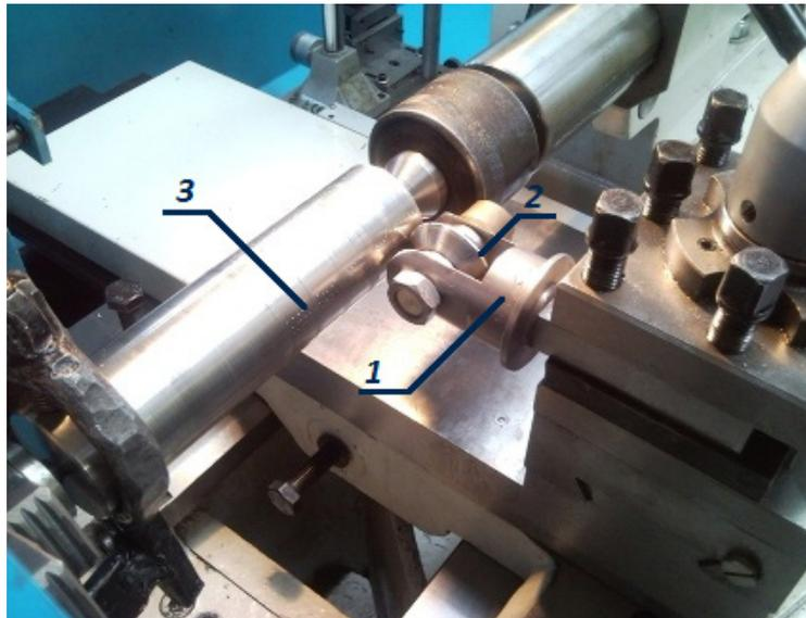
Fig. 1. The schema of burnishing rolling – pressuring process (BRP), 1 – burnished roller (BR-01), 2 – disk burnishing tool, 3 – outer cylindrical surfaces
