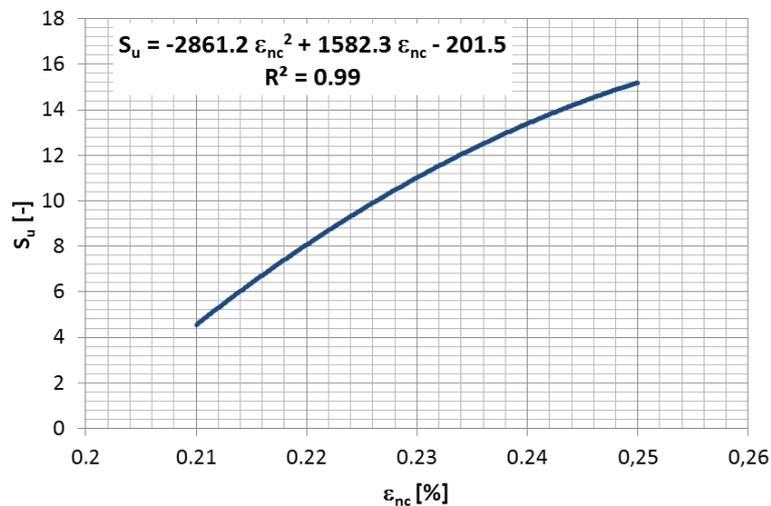
Fig. 5. The influence of the relative plastic deformation ( $\epsilon_{nc}$ ) on degree of relative strain hardening ( $S_u$ )
