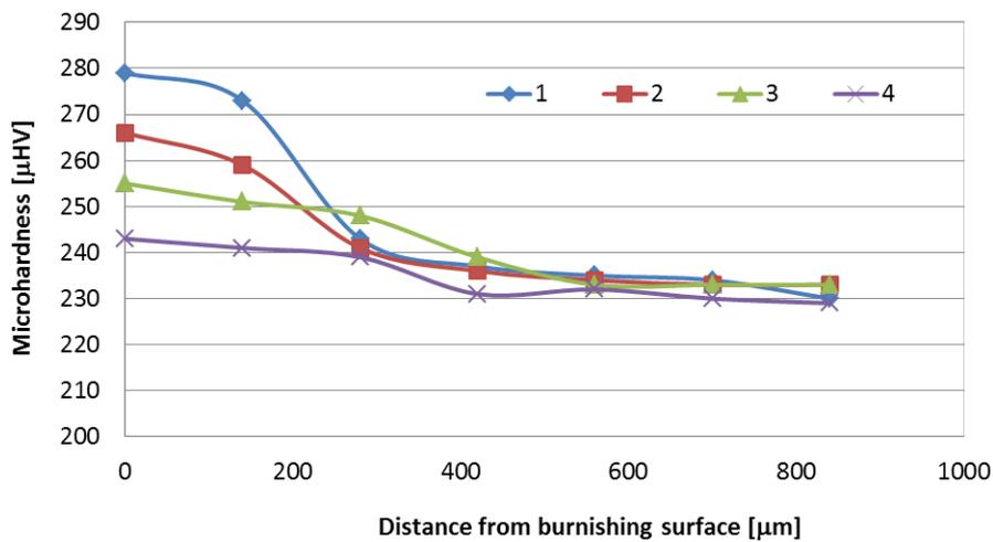
Fig. 4. Distribution microhardness on the distance from burnishing surface for the burnishing speed: 1 –  $v_n = 50$  m/min, 2 –  $v_n = 70$  m/min, 3 –  $v_n = 100$  m/min, 4 –  $v_n = 140$  m/min, for relative plastic deformation  $\epsilon_{nc} = 0.25\%$  for disk burnishing tool feed  $a_n = 1$  mm and feed  $f_n = 0.1$  mm/rev
