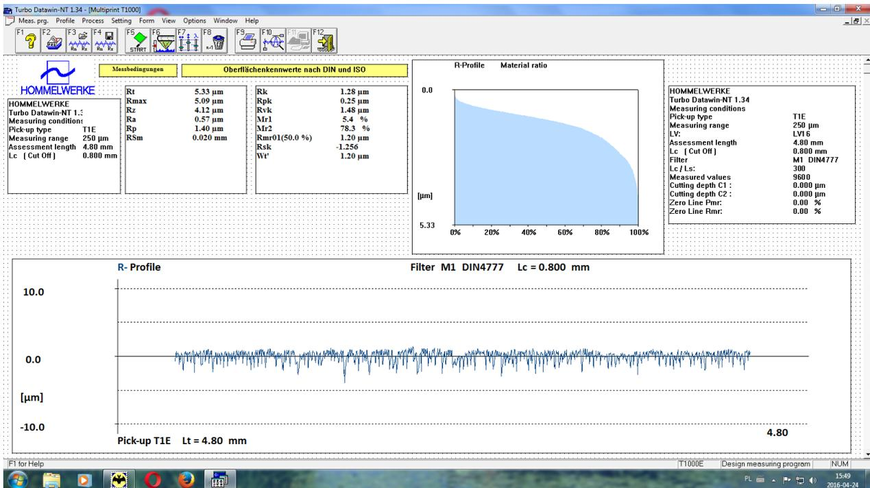
Fig. 2. The Abbott-Firestone curve and the profile roughness for relative plastic deformation  $\epsilon_{nc} = 0.25\%$  after burnishing rolling – pressuring process (BRP) for the samples No. 23 for stainless steel X2CrNiMo17-12-2 (316L) for disk burnishing tool feed  $a_n = 1$  mm and feed  $f_n = 0.1$  mm/rev and burnishing speed  $v_n = 70$  m/min
