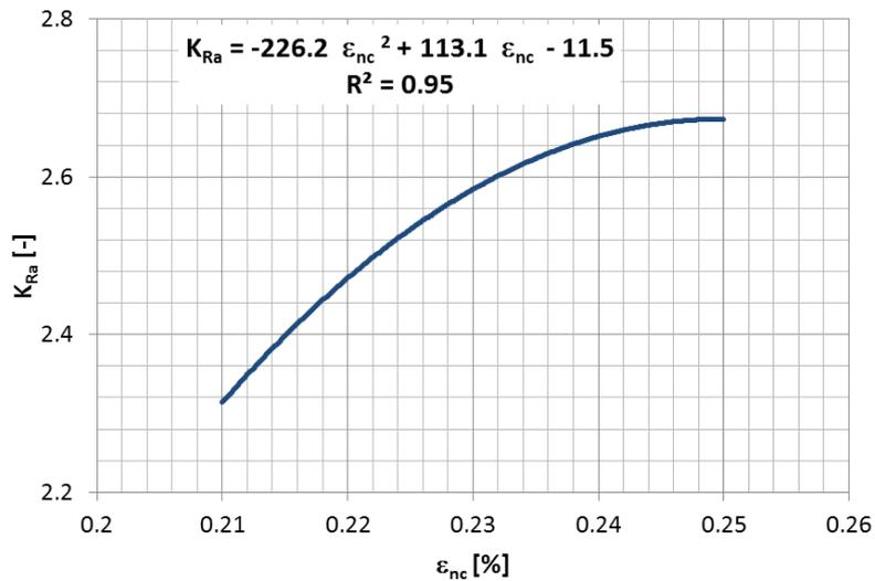
Fig. 3. The influence of the relative plastic deformation ( $\epsilon_{nc}$ ) on surface roughness reduction ratio ( $K_{Ra}$ ) after burnishing rolling – pressuring process (BRP)
