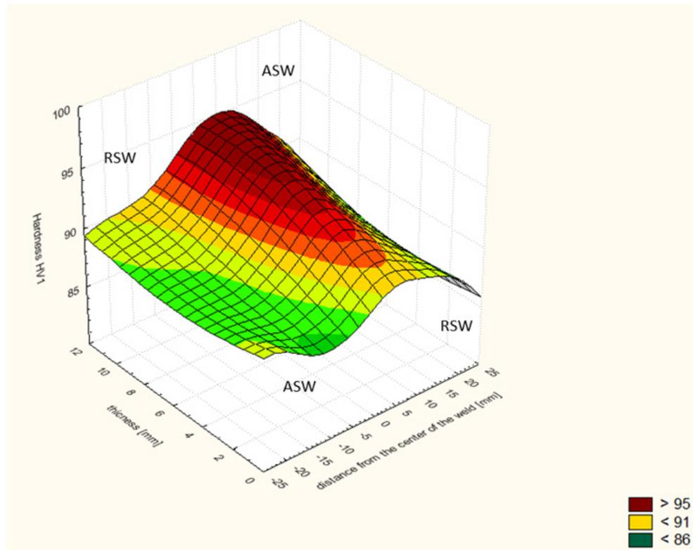
*Fig. 4. Hardness distribution in joint welded by tool with conical pin, ASW – Advancing Side of the Weld, RSW – Retreating Side of the Weld*
