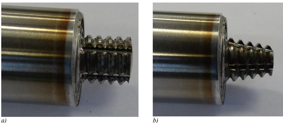
*Fig. 2. View of tools used for joining by FSW: a) with cylindrical pin, b) with conical pin*
