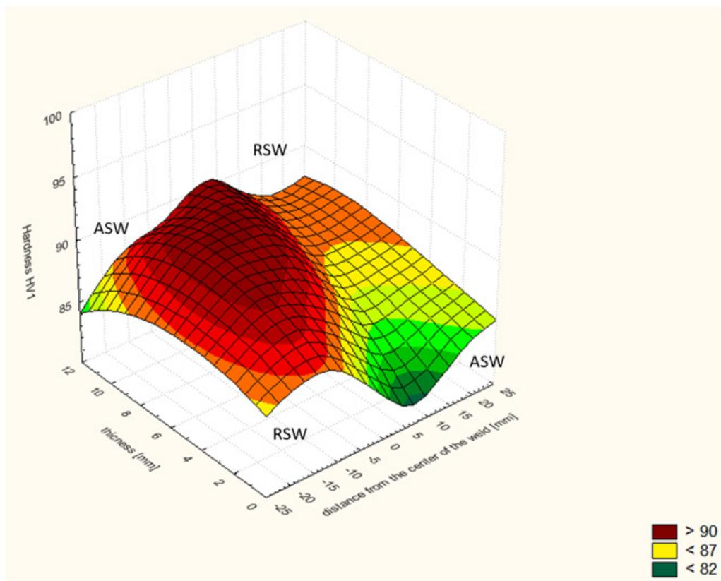
Fig. 3. Hardness distribution in joint welded by tool with cylindrical pin, ASW – Advancing Side of the Weld, RSW – Retreating Side of the Weld
