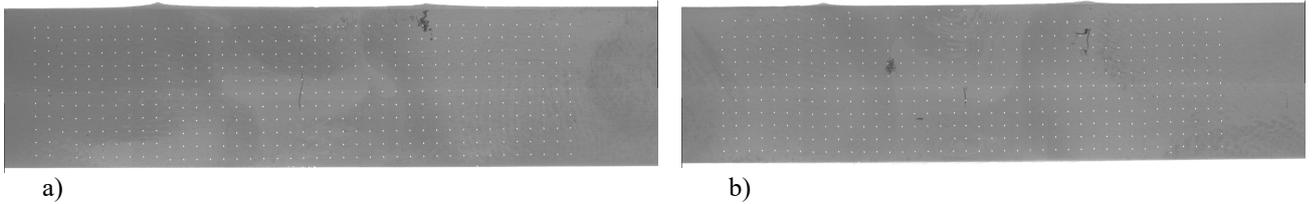
Fig. 2. The view of FSW welded specimens after hardness testing with visible measurement points: a) welded by cylindrical tool, b) welded by conical tool
