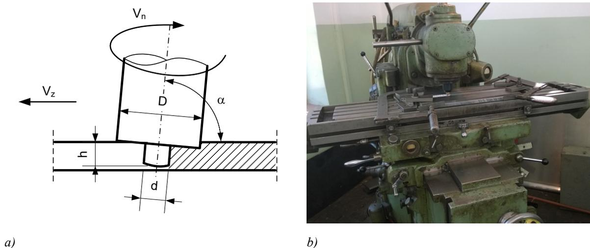
Fig. 1. The diagram of FSW (a) and view of stand used in research (b)
