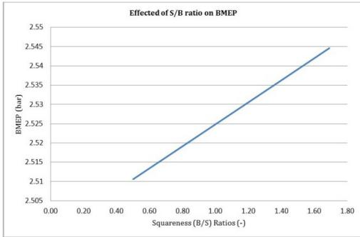
Fig 4(e). Brake Mean Effective Pressure from AVL BOOST simulation
