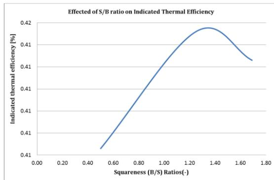
*Fig. 4(a). Indicated thermal efficiency from AVL BOOST simulation*
