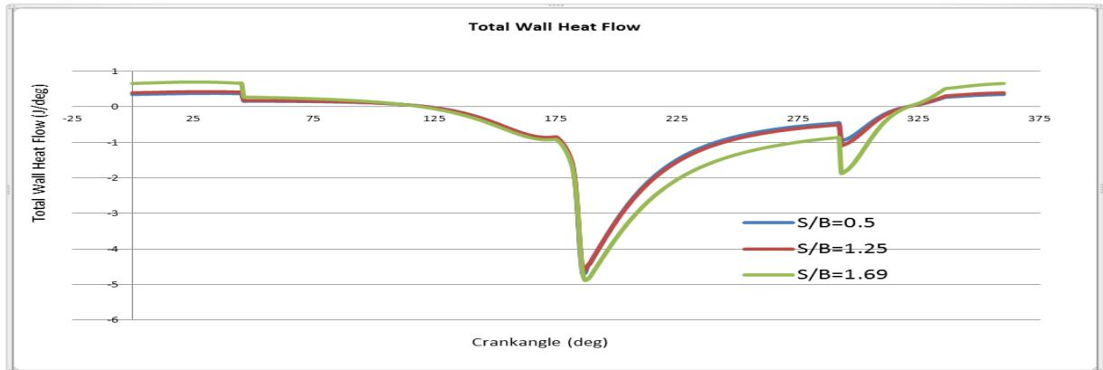
*Fig 3. Wall heat flow from AVL BOOST simulation*
