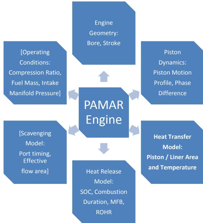
Fig. 1. Numerical model input data flow
