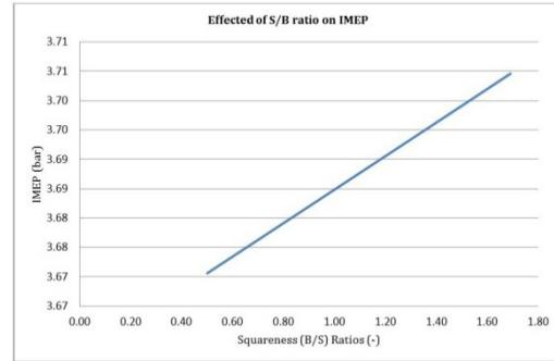
Fig 4(f). Indicated Mean Effective Pressure from AVL BOOST simulation
