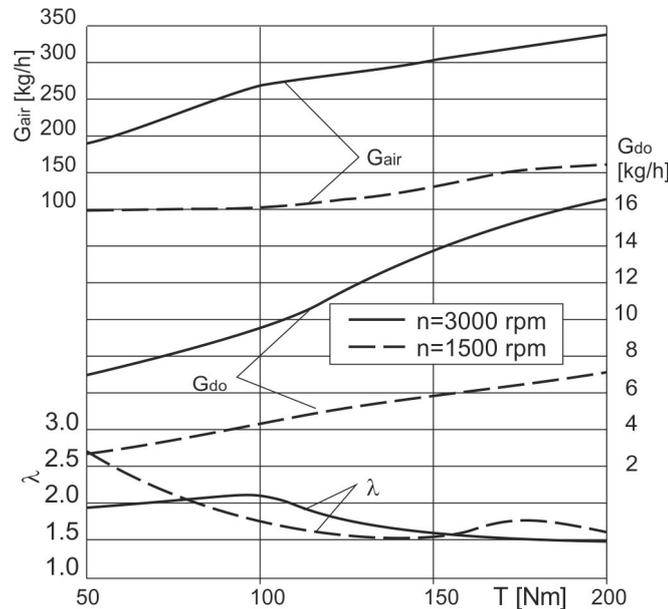
Fig. 1. A course of the change in the mass of the drawn air, the consumption of fuel and the  $\lambda$  ratio as a function of the engine load at  $n = 1500$  and  $n = 3000$  rpm for an ADCR engine
