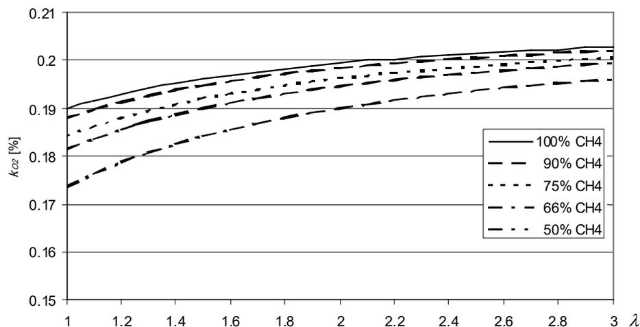
Fig. 6. The changes in the concentration of oxygen in the gas and air mixture for various shares of methane in biogas depending on the  $\lambda$  ratio
