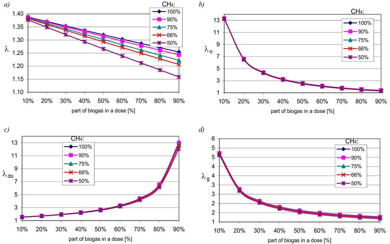
Fig. 4. The impact of the share of biogas in the dose powering the engine for fuels of varying methane content at  $n = 3000$  rpm and  $T = 200$  Nm on the ratios: a)  $\lambda$ , b)  $\lambda_o$  b)  $\lambda_{do}$  b)  $\lambda_g$
