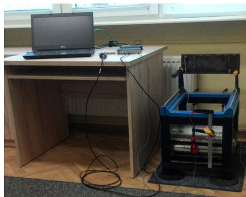
*Fig. 1. Test stand for testing of welded joints with use the vibration methods*
