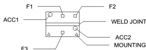
*Fig. 2. Schematic diagram showing the arrangement of accelerometers (ACC1, ACC2), places of strokes (F1, F2, F3) and plates mounting places in the holders (Δ)*
