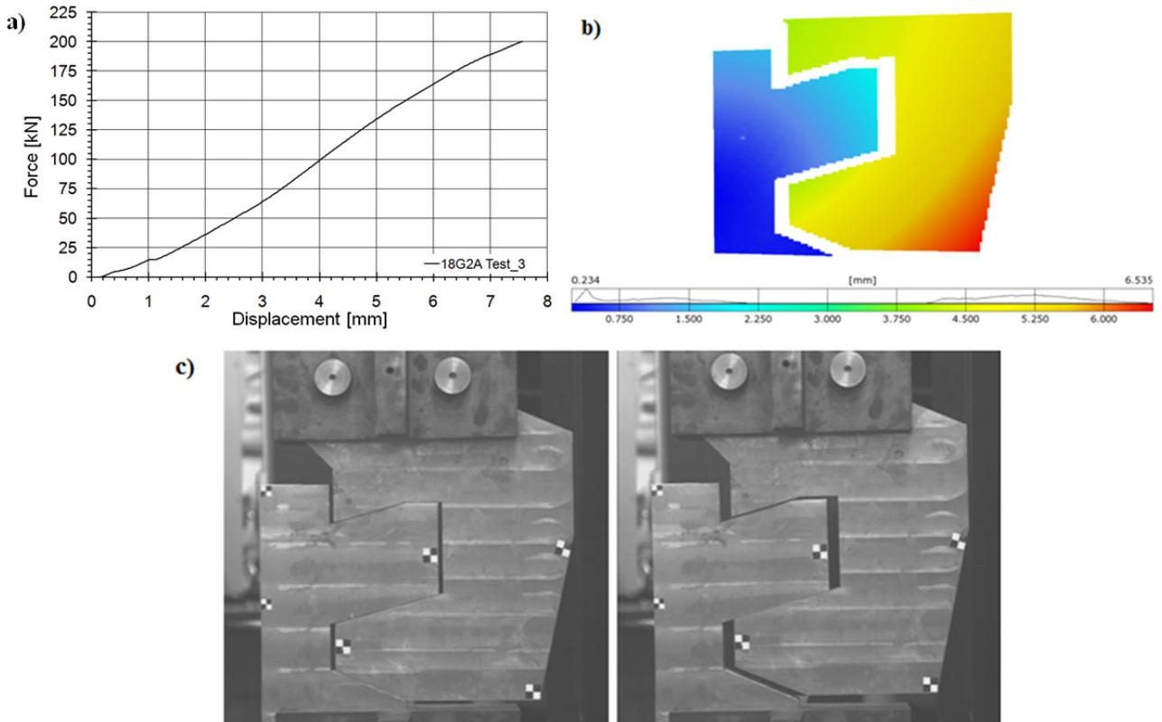
Fig. 7. Selected results of stand test: a) force – displacement curve, b) displacement map of the hook-shape connector, c) photographs of the connector deformations before and during the load test
