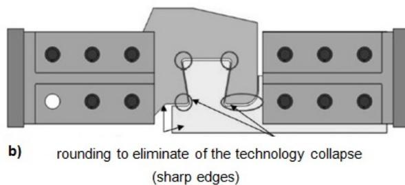
Fig. 11. View of numerical model mapping a modified shape of the lock connectors – dovetail joint without sharp edges
