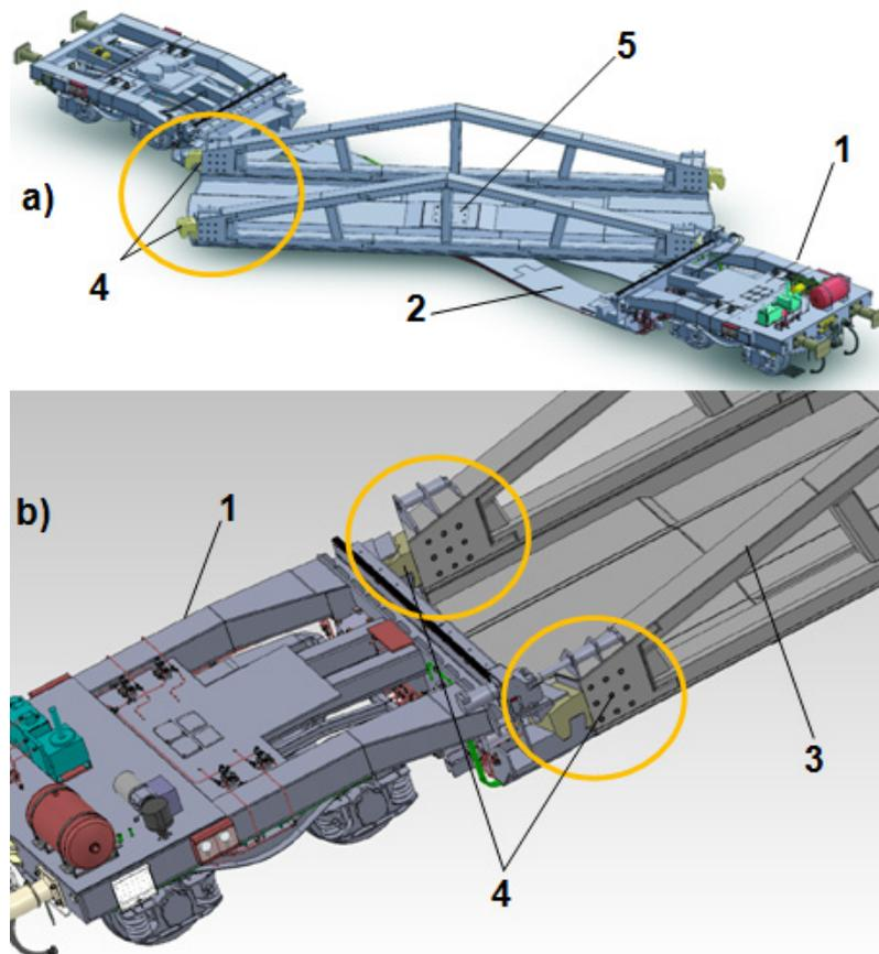
Fig. 1. Prototype version of the wagon [6, 7] with: a) open loading platform, b) closed loading platform with the view of lock components: 1 – over-bogie part of the wagon, 2 – lowered fixed frame of the wagon, 3 – side of the moving loading platform, 4 – hook shape locks with the support area, 5 – central node of the rotatable platform
