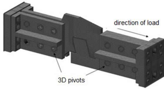
Fig. 8. FE models mapping two different shapes of lock connectors (as in the experimental tests): initial hook-shape lock
