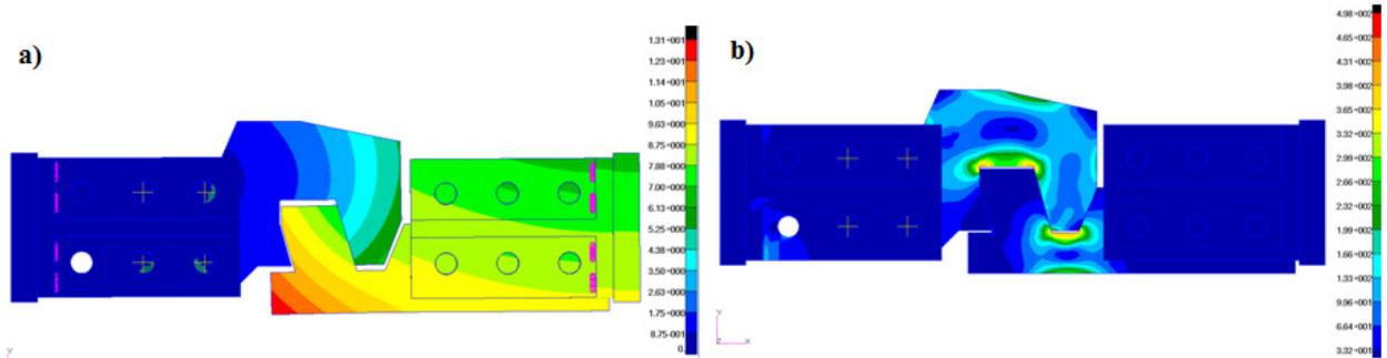
Fig. 9. Results maps for Variant I of load: a) displacement –  $V_{max} = 12 \text{ mm}$ , b) H-M-H stresses –  $\sigma_{max} = 365 \text{ MPa}$
