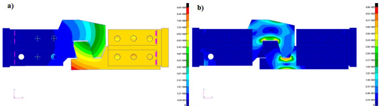
Fig. 10. Results maps for Variant II of load: a) displacement –  $V_{max} = 8.5 \text{ mm}$ , b) H-M-H stresses –  $\sigma_{max} = 350 \text{ MPa}$
