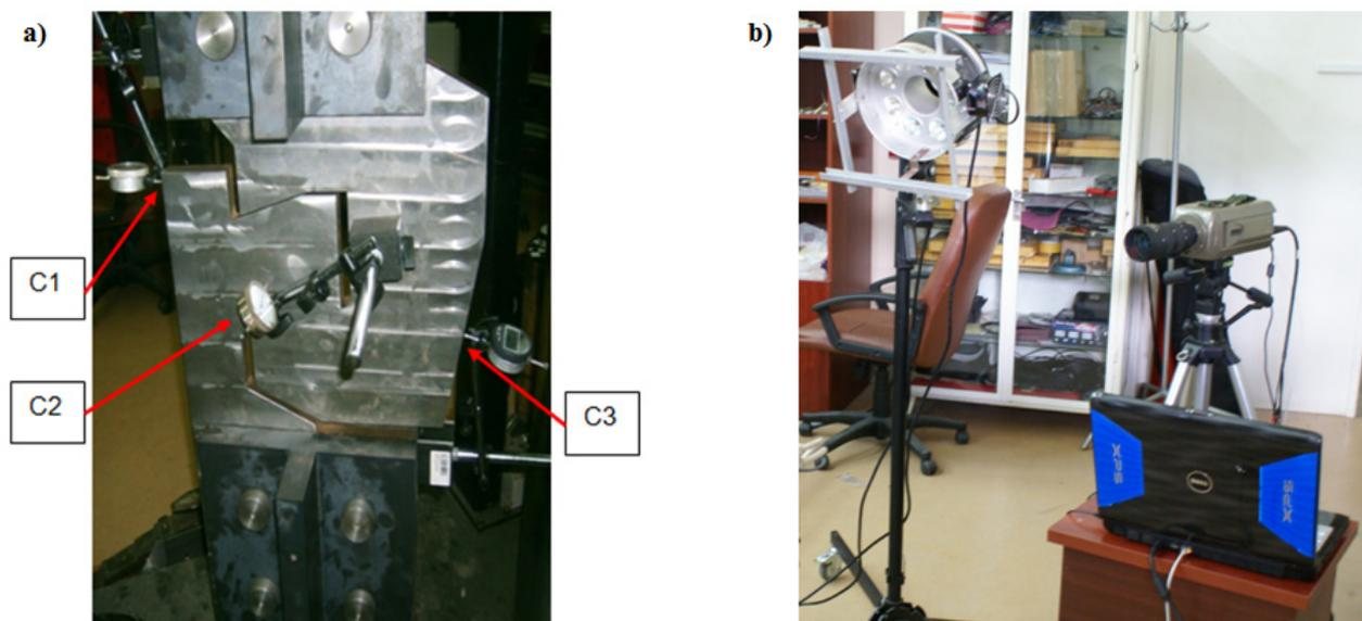
Fig. 6. Photos of the tested components of the side lock and the test stand view with INSTRON SATEC machine: a) hook-shaped connector with the measuring equipment, b) additional stand equipment: black-and-white camera to high-speed and high-resolution images Phantom V12 with halogen lamps
