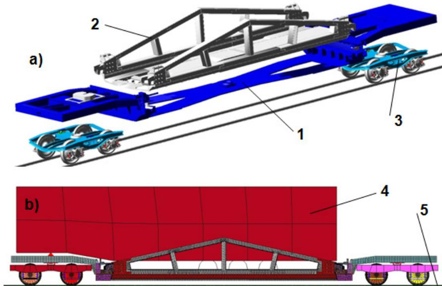
Fig. 2. A View of 3D numerical model [3, 8]: a) multibody model with main subsystems, 1 – chassis frame of the wagon, 2 – rotatable platform, 3 – Y25 type bogie with the suspension [12]; b) FE model of the complete wagon for dynamic simulation [3, 8], 4 – semitrailer with load, 5 – railway track
