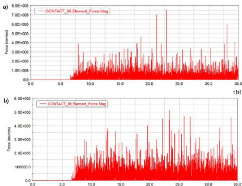
Fig. 3. The chart of contact forces in the selected lock as a result of 3D multibody analysis: a) during passage of the wagon on the curved track at a speed of 60 km/h, b) during passage of the wagon on the curved track at a speed of 80 km/h [12]
