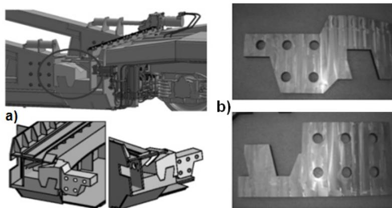
Fig. 5. Views: a) side lock area between rotatable platform and over bogie part of the intermodal wagon, b) separated hook-shaped connector prepared for tests
