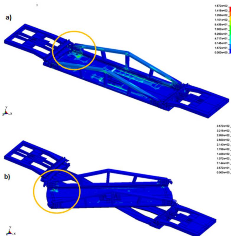
Fig. 4. FE numerical result – HMM stress of the lock components areas in the special wagon with  $1.95 \cdot Q$  load and: a) closed platform after unblocking the side locks –  $\sigma_{max} = 157$  MPa, b) opened platform with load and rotated by an angle of  $50^\circ$  –  $\sigma_{max} = 357$  MPa
