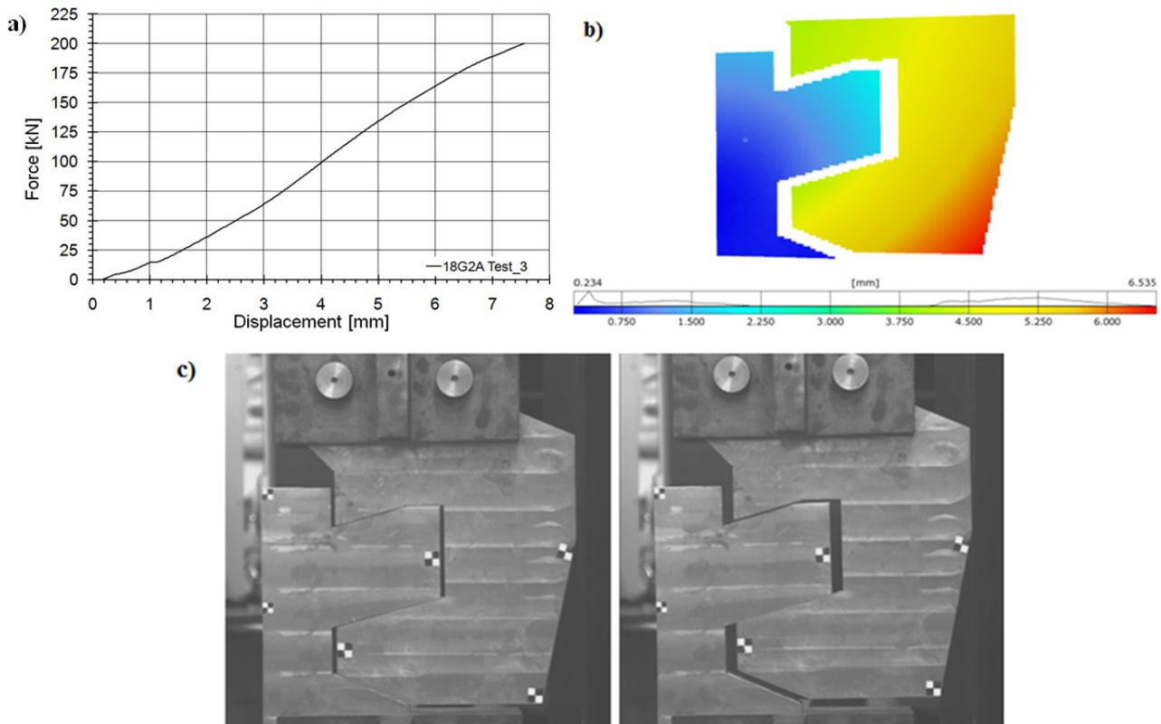
Fig. 7. Selected results of stand test: a) force – displacement curve, b) displacement map of the hook-shape connector, c) photographs of the connector deformations before and during the load test
