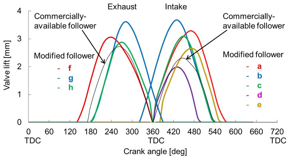
Fig. 3. Valve opening period and valve lift
