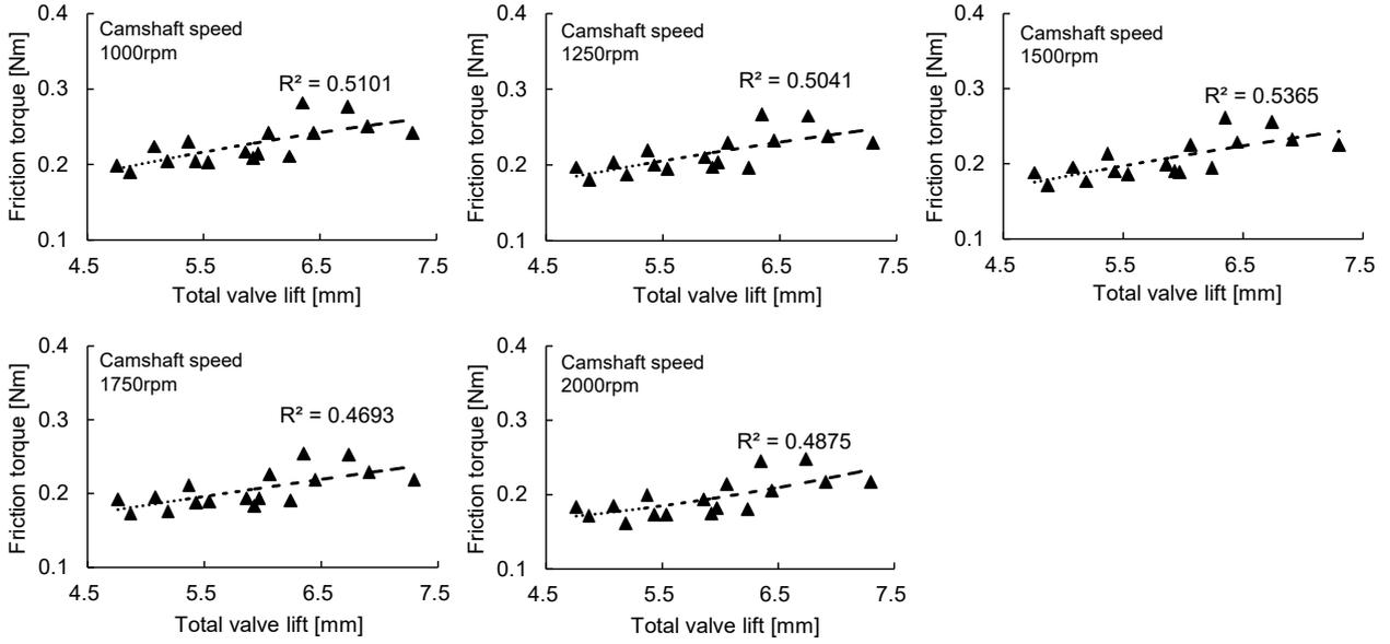
Fig. 6. Friction torque vs. total valve lift
