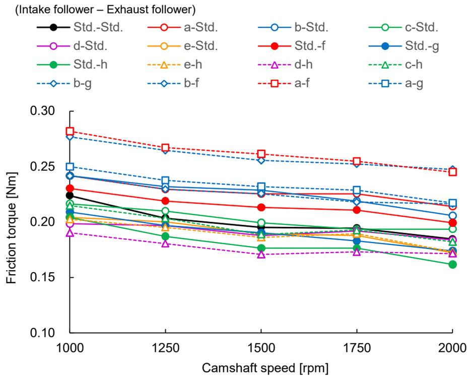
Fig. 4. Friction torque in various combinations of intake and exhaust followers
