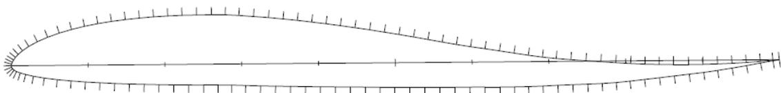
Fig. 5. Airfoil cross-section modification of S5010
