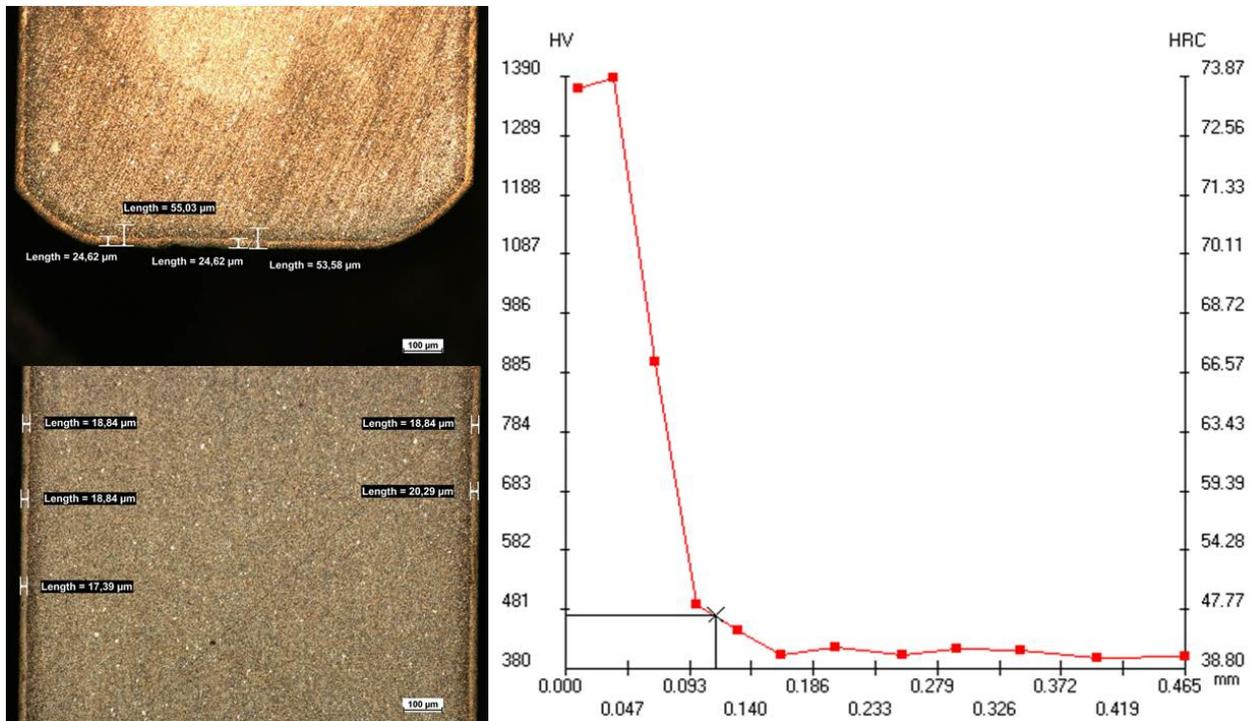
Fig. 1. Microstructure of nitrided piston ring 1-2, x100 (on the left side) and hardness distribution HV0.1 from surface to core (on the right side)
