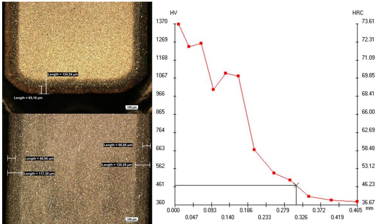
Fig. 4. Microstructure of nitrided piston ring 1-32,  $\times 100$  (on the left side) and hardness distribution HV0.1 from surface to core (on the right side)
