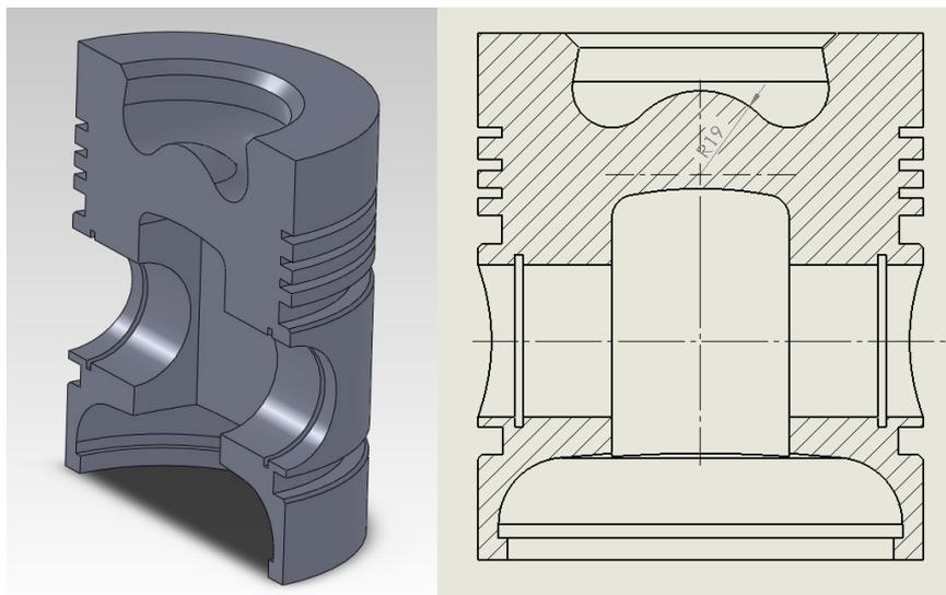
Fig. 6. The shape of the chamber „55c”
