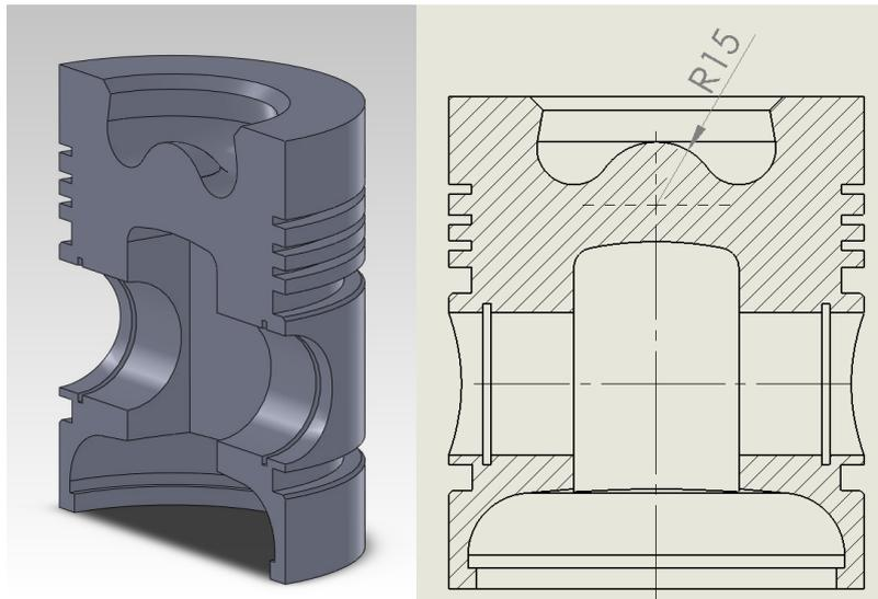
Fig. 5. The shape of the chamber „55b”
