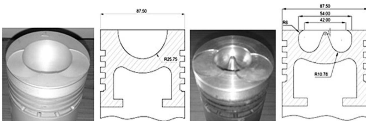
Fig. 1. Examples of studied combustion chambers [1]
