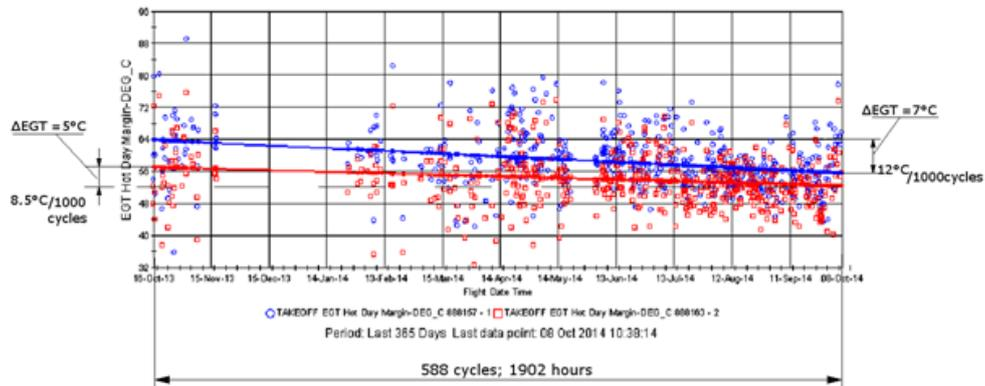
*Fig. 3. EGTM decrease of the 100 kN thrust engines installed on medium range aircraft (Airline approval)*
