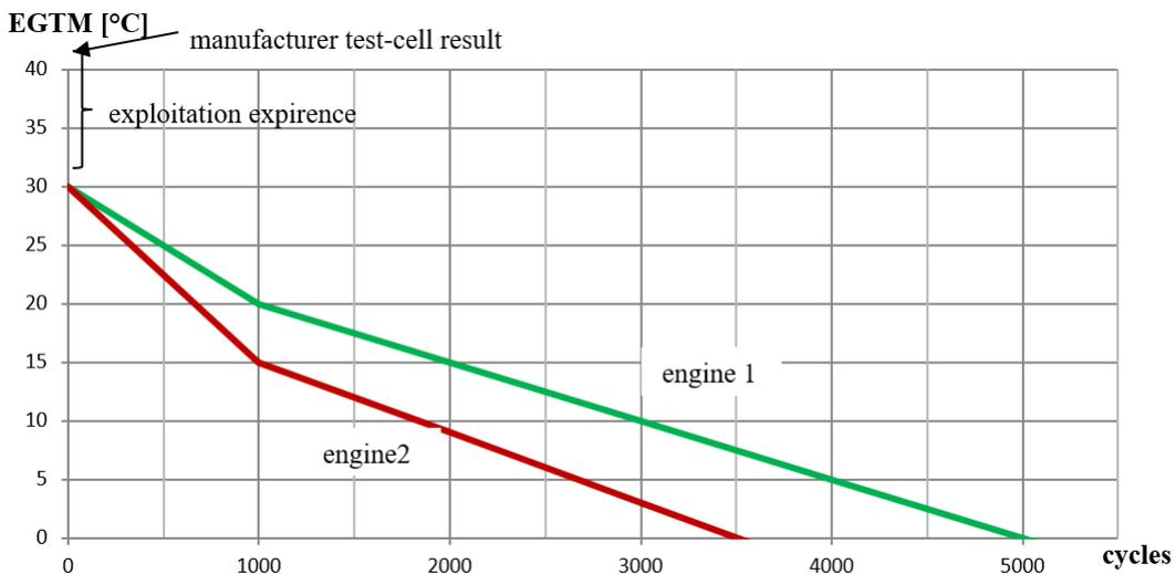
Fig. 2. Expected time on wing for two engines delivered to the operator from overhaul
