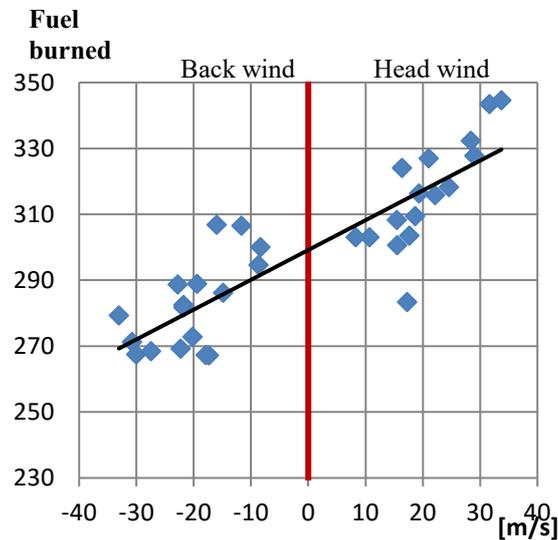
*Fig. 4. Aircraft fuel consumption per 100 km on certain depending on axial component of the jet stream*
