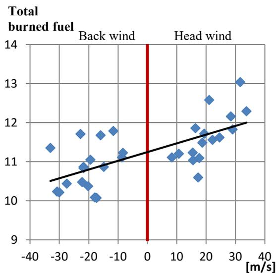
*Fig. 5. Total aircraft fuel consumption on certain route depending on axial component of the jet stream*
