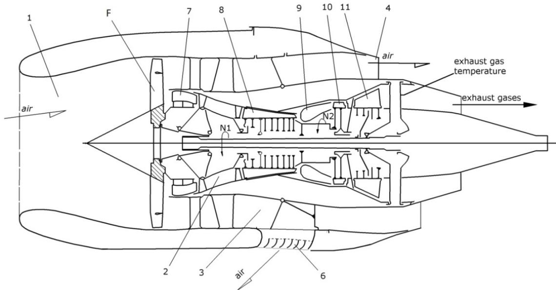
*Fig. 1. Schematically presented basic features of modern turbofan engine: 1 – Engine inlet, F – Fan, 2 – internal duct, 3 – external duct, 4 – Air exhaust, 5 – Exhaust nozzle, 6 – Thrust reverser vanes, 7 – Low pressure compressor, 8 – High pressure compressor, 9 – Combustion chamber, 10 – High pressure turbine, 11 – Low pressure turbine, N1 – Low pressure rotor speed, N2 – High pressure rotor speed*
