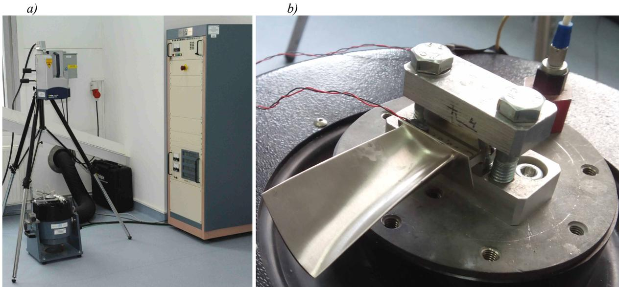
Fig. 1. View of the vibration system (a) and blade fixed to the head of vibrator (b)
