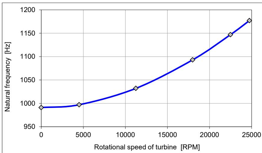
Fig. 5. Natural frequency of the blade (mode I) as a function of the rotational speed of turbine (model no. 3)
