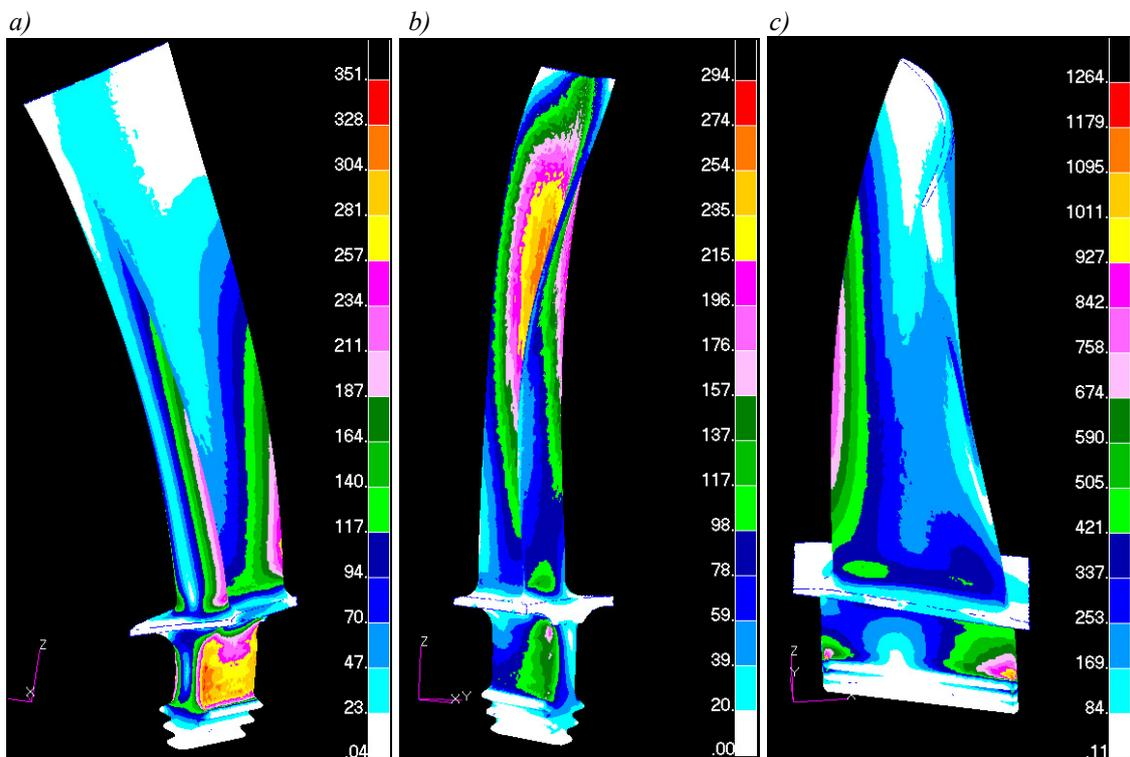
Fig. 4. Von Mises stress distributions for the turbine blade during first (a), second (b) and third (c) mode of free vibrations (for blade amplitude close to 1 mm, blade no. 3,  $n=0$  RPM)
