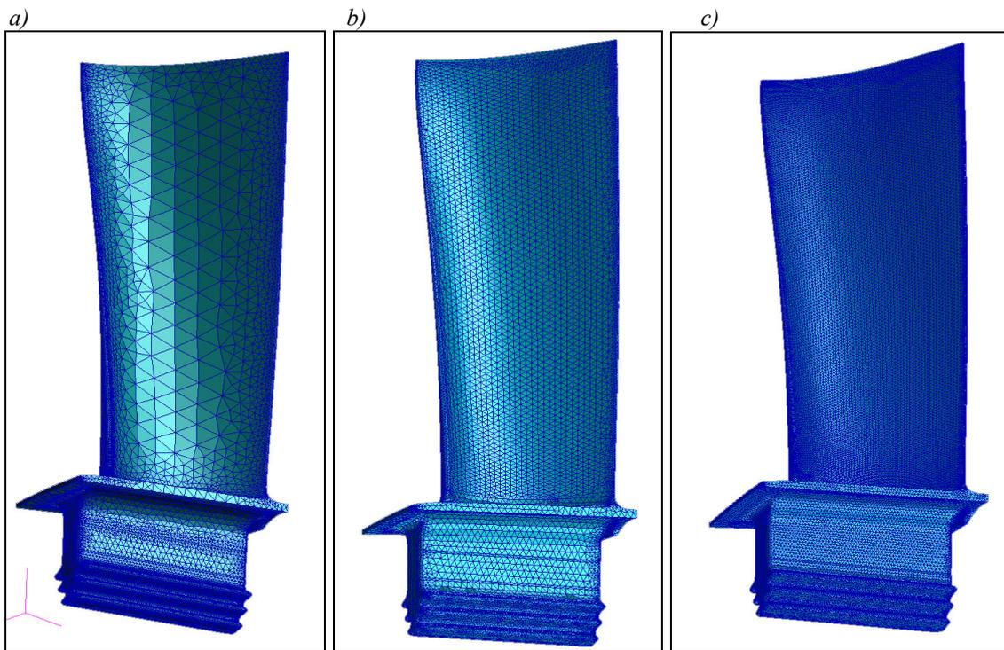
Fig. 3. Numerical models of the blade with different mesh size. Model no. 1 (a), no. 2 (b) and no. 4 (c)
