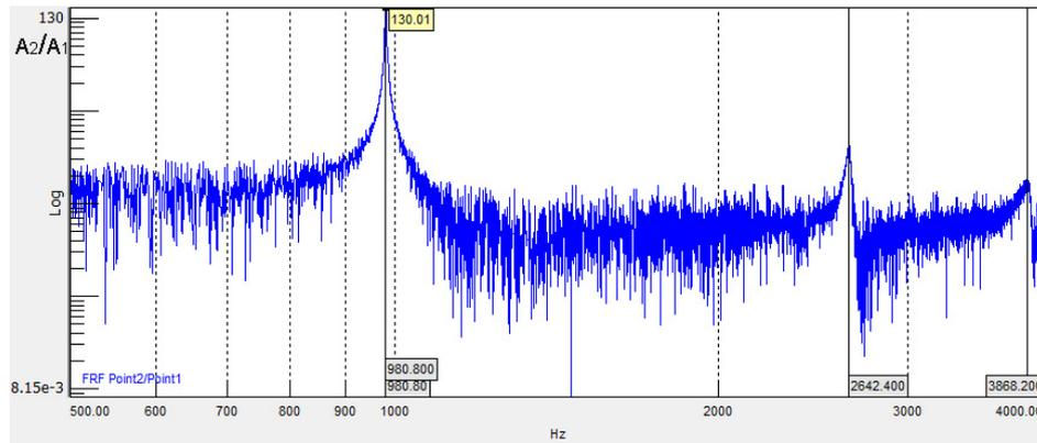
Fig. 2. Amplitude-frequency characteristic for investigated turbine blade
