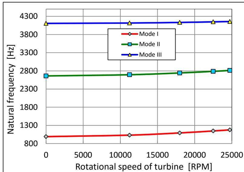
Fig. 6. Natural frequencies of the blade for first, second and third mode of vibrations as a function of rotational speed of turbine (model no. 3)
