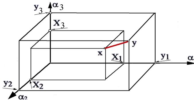
Fig. 4. The Euclidean metric transport distance between outgoing place  $x(x_1, x_2, x_3)$  and delivery place  $y(y_1, y_2, y_3)$ , defined in the three dimensional space  $D_3$
