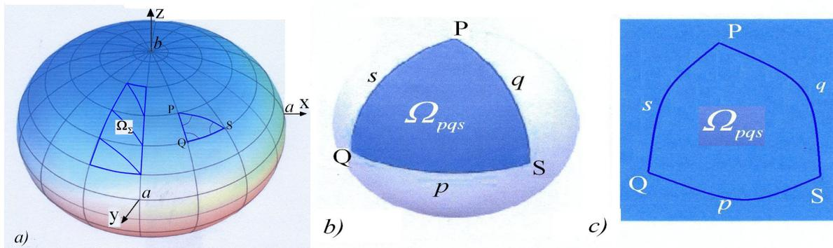
Fig. 7. Elliptical triangle with apex PQR lying on the Earth Ellipsoid as a non-Euclidean metric road transport space: a) triangle on the Earth Ellipsoid, b) approximation of the elliptical triangle, c) a view of elliptical triangle reduced to the plane
