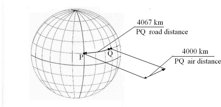
Fig. 8. Differences between metric transport road distance PQ on the Earth surface and metric transport air distance for the same places P and Q
