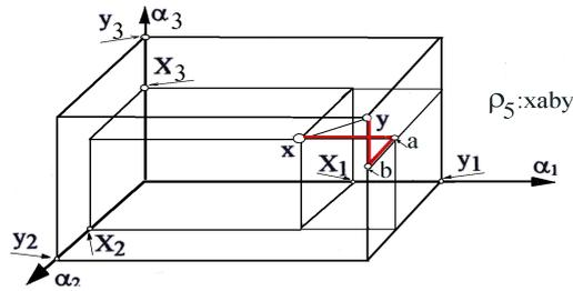
Fig. 10. The non-Euclidean modular (Taxi Car) metric transport distance between outgoing place  $x(x_1, x_2, x_3)$  and delivery place  $y(y_1, y_2, y_3)$ , defined in the two dimensional space  $D3: X=\alpha_1 \times \alpha_2 \times \alpha_3$
