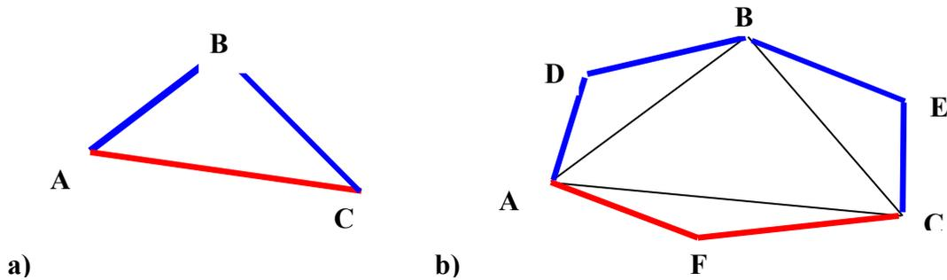
Fig. 5. Triangles in transport metric space D2: a) On the left- the Euclidean triangle with apexes A, B, C in the classical Euclidean metric transport presents way from A direct to B or through the point C; b) On the right- the polygon ADBECF as the triangle in non-Euclidean metric transport space, where way from A to B leads only through the point D
