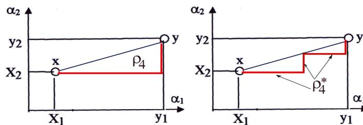
Fig. 9. The non-Euclidean modular (Taxi Car) metric transport distance between outgoing place  $x(x_1,x_2)$  and delivery place  $y(y_1,y_2)$ , defined in the two dimensional space  $D2: X=\alpha_1 \times \alpha_2$
