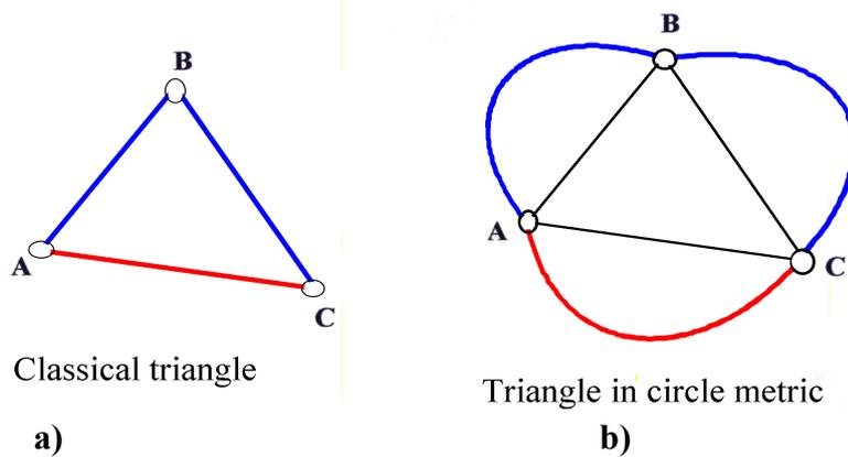
Fig. 6. Triangles in transport metric space D2: a) On the left- the Euclidean triangle with apexes A, B, C in the classical Euclidean metric transport; b) On the right- the triangle ABC in non-Euclidean metric transport space, where distance from A to B leads only through the bow way, similarly distance from B to C leads only through the bow
