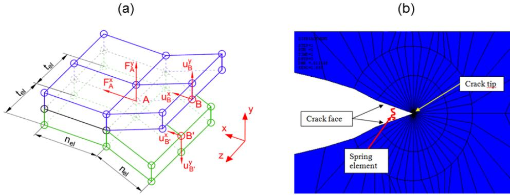
Fig. 3. Circumferential crack position in investigated boiler with flat end plate- (a), Finite element mesh of structure around crack tip- (b)
