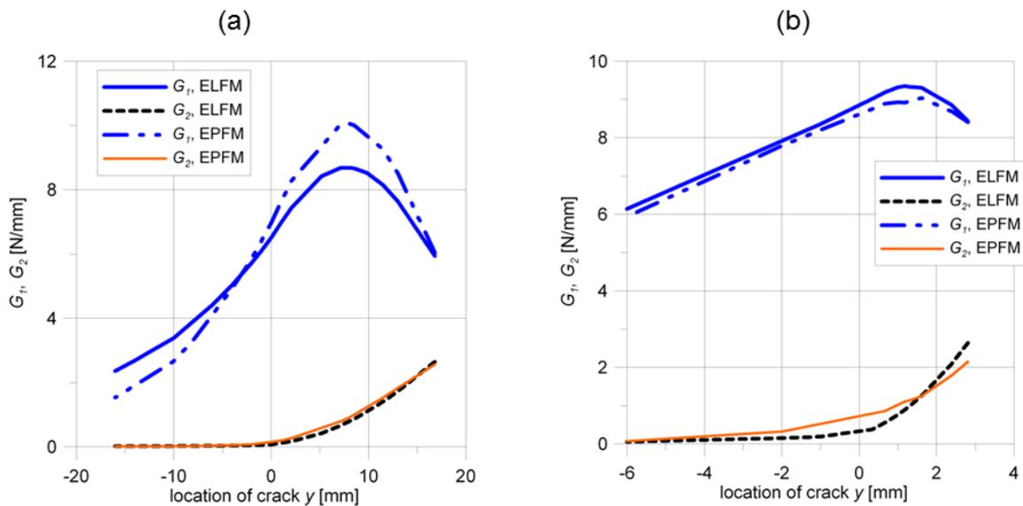
Fig. 5. Strain energy release rate  $G$  for different location of cracks, 2D axisymmetric model, crack length 4.216 mm, optimal shape of stress relieve groove (a), not-optimal shape (b) – results for 16Mo3 steel
