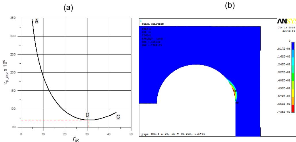
Fig. 2. Distribution of maximum equivalent plastic strains along line AC (see Fig.1b) – (a); distribution of equivalent plastic strains in analysed structure for optimum value of  $r_{ik} = 32.0$  (point D) – (b)
