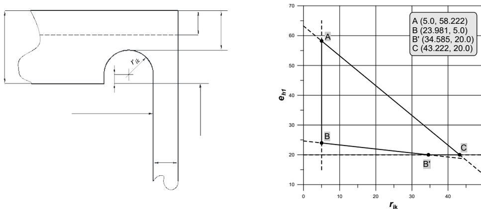
Fig. 1. Stress relieve groove of circular shape (a); admissible area for groove radius and minimum endplate thickness calculated for boiler:  $\text{Ø}406,4 \times 20$  made from 16Mo3 steel
