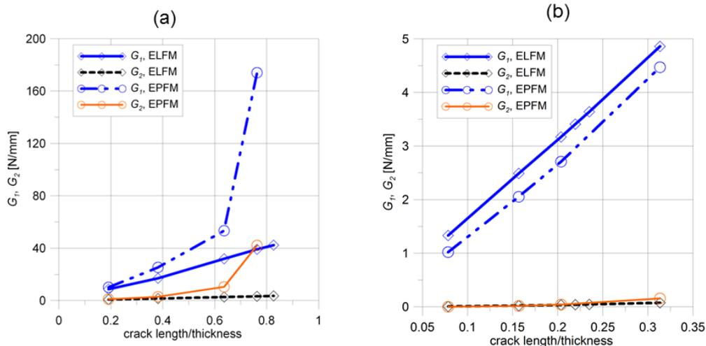
Fig. 6. Strain energy release rate  $G_1$  for different crack length, 2D axisymmetric model,  $y = 8.04$  mm, optimal shape of relief groove: steel 16Mo3 – (a); steel s235JR – (b)
