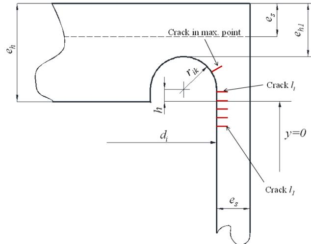
Fig. 4. Considered positions for cracks
