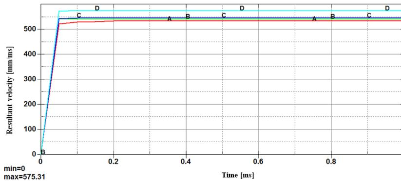
Fig. 8. Time-velocity graph for fragments originating from opposite end – top layer
