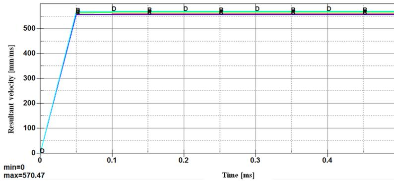
Fig. 6. Time-velocity graph for fragments originating from opposite end – top layer
