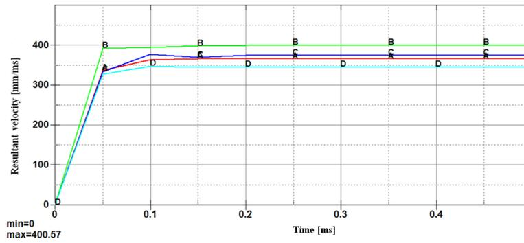
Fig. 5. Time-velocity graph for fragments originating from detonation point – top layer
