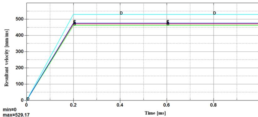
Fig. 14. Time-velocity graph for fragments originating from right end – top layer
