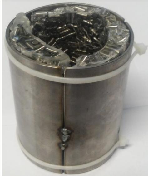
Fig. 1. Cylindrical fragmentation warhead
