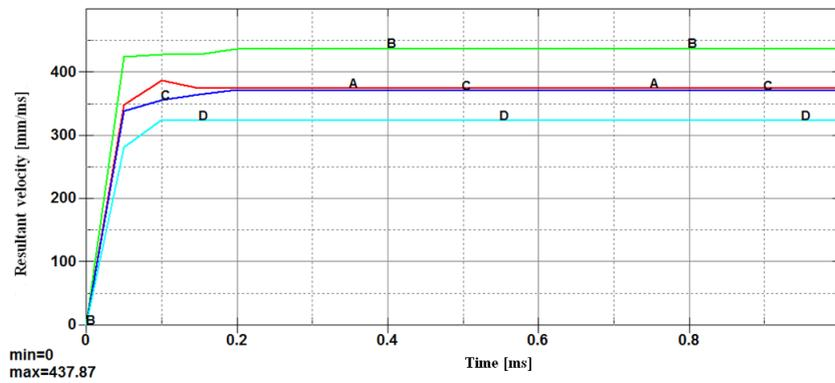
Fig. 7. Time-velocity graph for fragments originating from detonation point – top layer
