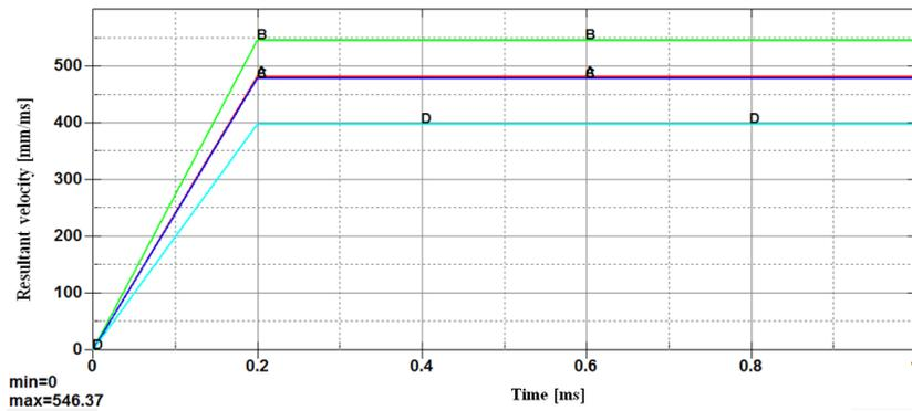
Fig. 13. Time-velocity graph for fragments originating from left end – top layer
