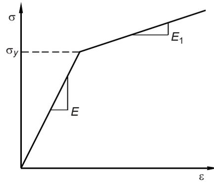
Fig. 7. Bilinear model of an elastic-plastic material,  $E_1 = 0.1 E$
