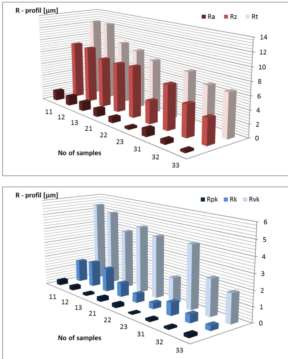
Fig.4. The parameters of the surface roughness and parameters of the material ratio curve after ballizing process for samples refer with Tab. 1
