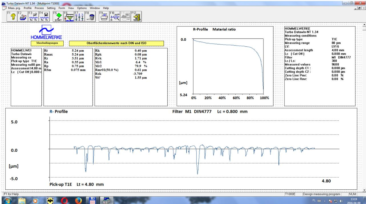
Fig. 3. The material ratio curve and the profile roughness after ballizing process for relative plastic deformation  $\epsilon_{np} = 1.4\%$  (sample No. 23)
