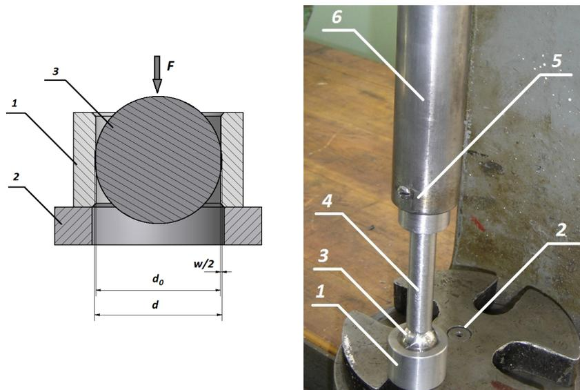
Fig. 1. The schema of ballizing process,  $d$  – outer diameter of the ball,  $d_0$  – diameter inner tube before burnishing,  $w$  – reduction ratio, 1 – tube hole, 2 – basis of hydraulic press PH-16, 3 – ball, 4 – guide-pin ball, 5 – mounting socket, 6 – punch of hydraulic press PH-16
