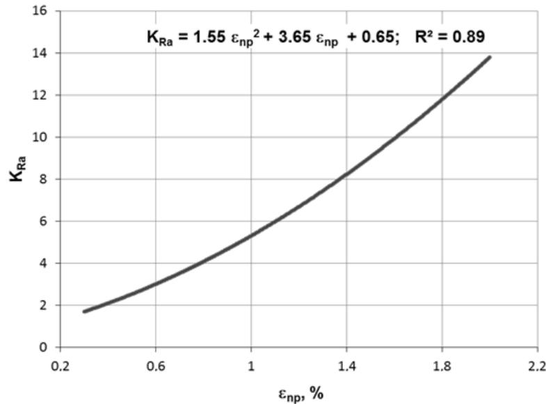
Fig. 5. The influence of the relative plastic deformation ( $\epsilon_{np}$ ) on the surface roughness reduction rate ( $K_{Ra}$ )
