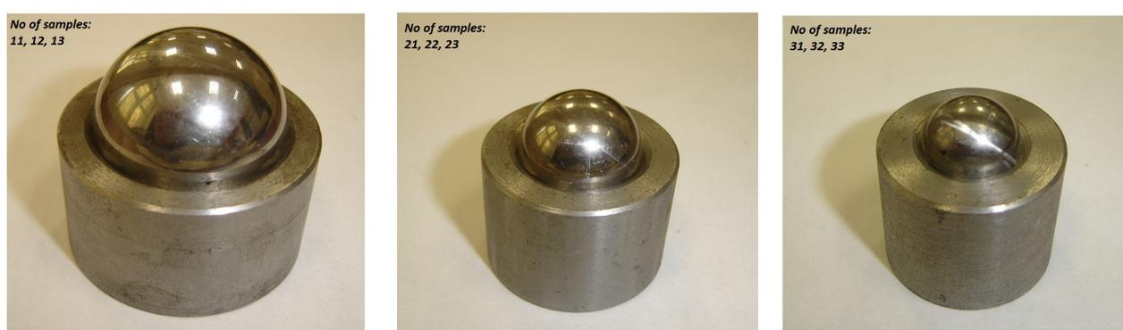
Fig. 2. The samples and ball burnishing used for ballizing process
