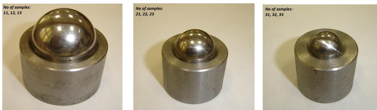
Fig. 2. The samples and ball burnishing used for ballizing process
