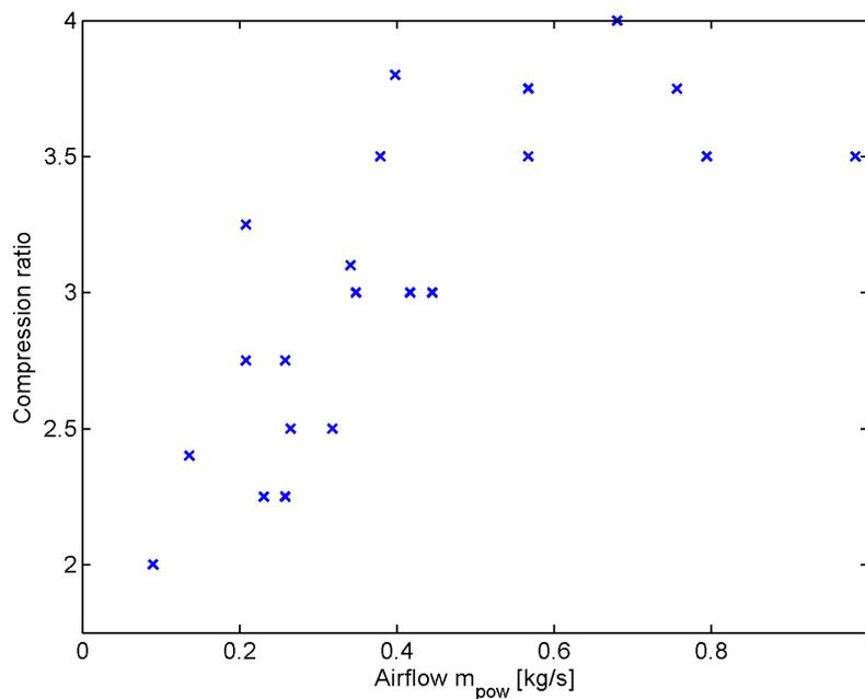
Fig. 2. Centrifugal compressor rotor database (manufacturer Garret)
