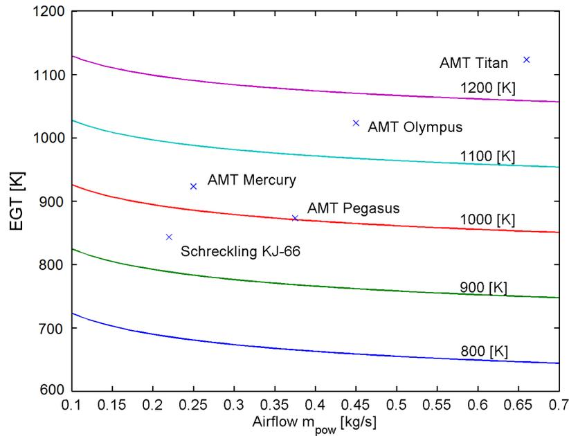
Fig. 7. Identification of microgasturbine exhausts gas temperature
