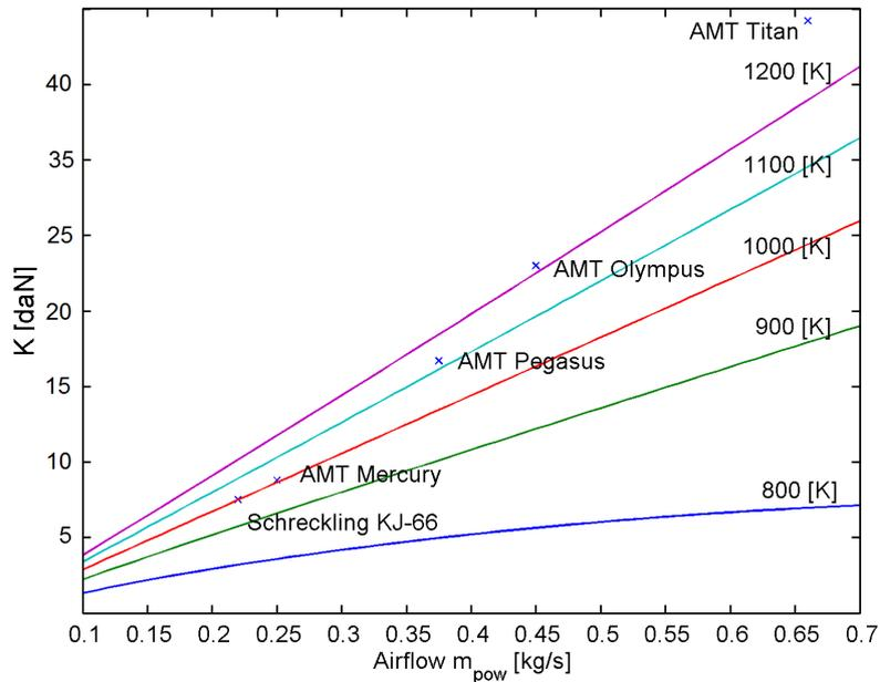
Fig. 9. Identification of microgasturbine thrust
