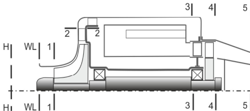
Fig. 6. Microgasturbine turbojet engine layout: WL-1 – inlet, 1-2 – compressor, 2-3 – combustor, 3-4 – turbine, 4-5 – exhaust nozzle
