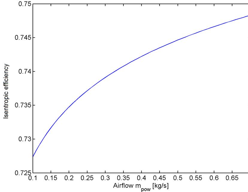
Fig. 3. Single centrifugal stage efficiency for microgasturbine engines
