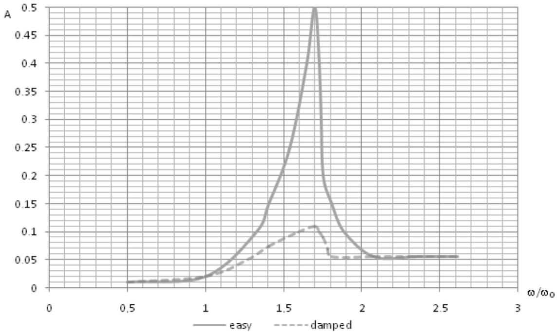
Fig. 5. The amplitude of forced vibration of harmonic oscillator in the dependence from of force input function frequency
