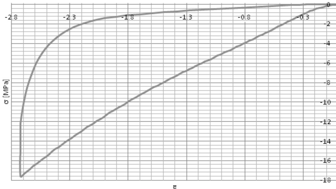
Fig. 4. Characteristic  $\sigma = f(\varepsilon)$  the grid elastomer of natural rubber – free grip
