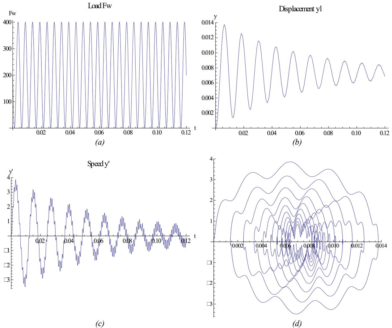
Fig. 7. Result analyse for initial conditions:  $t_p = 0$ ,  $t_k = 0.12$  s,  $T = 0.001$  s,  $C_1 = 0.9$ ,  $C_{01} = 5$
