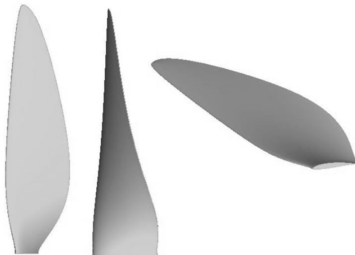
Fig. 9. Geometry of propeller blade designed for light, high altitude unmanned aerial vehicle
