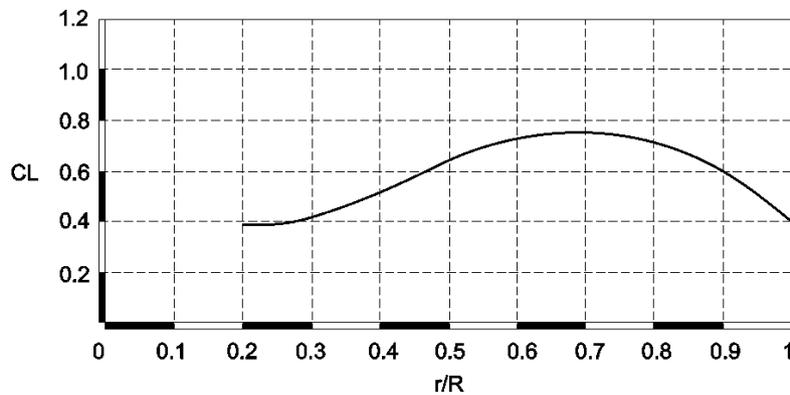
Fig. 8. Optimal shape of lift coefficient (CL) distribution curve for blade propeller intended for an experimental high altitude airplane
