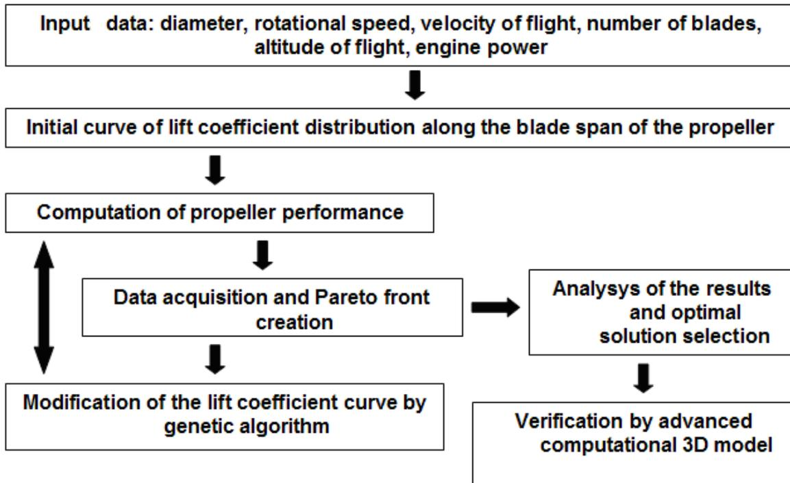
Fig. 1. Flowchart of calculation procedure supported by genetic algorithm method
