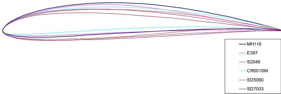
Fig. 2. Shapes of airfoils selected for analysis
