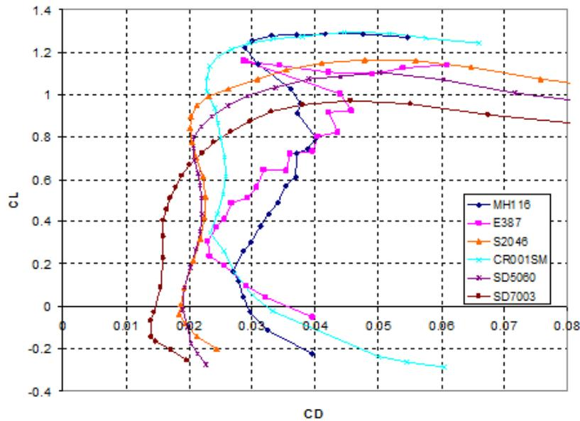
Fig. 3. Lift coefficients ( $CL$ ) versus Drag coefficients ( $CD$ ) characteristics of selected profiles for 0.75 radius of propeller blade cross section in high altitude flight condition (18000 metres), Reynolds number 70000, Mach number 0.4
