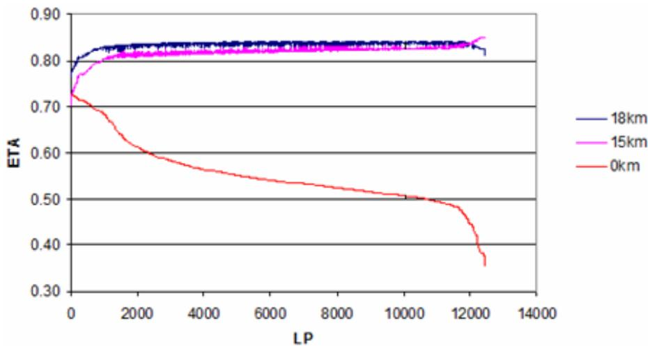
Fig. 5. Efficiency of propeller (ETA) for different variants (LP) of propeller design for three flight altitudes 0, 15000, 18000 metres
