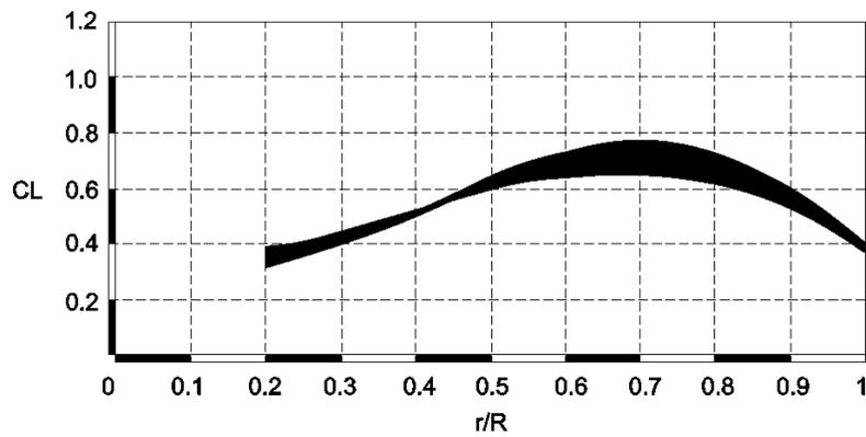
Fig. 7. Typical shapes of lift coefficient (CL) distribution curves for field of solutions marked in Fig. 6
