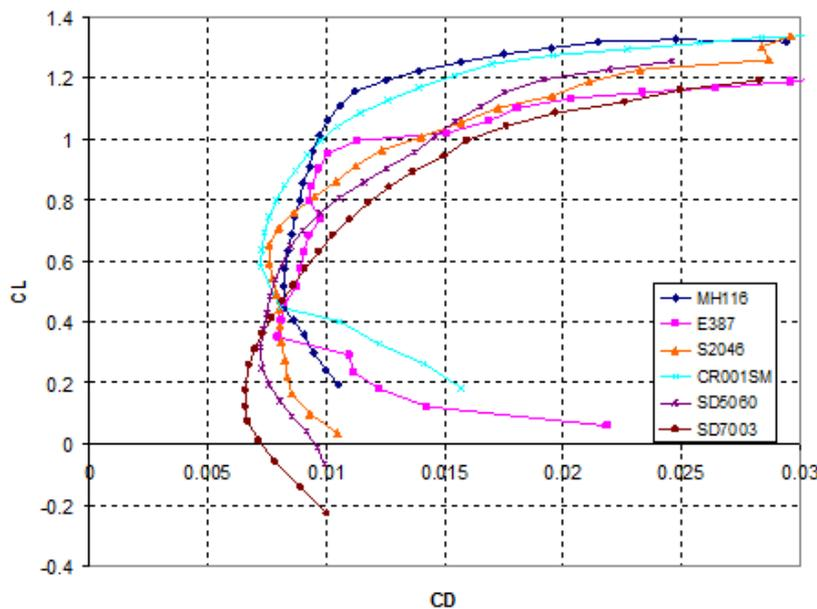
Fig. 4. Lift coefficients ( $CL$ ) versus Drag coefficients ( $CD$ ) characteristics of selected profiles for 0.75 radius of propeller blade cross section in low altitude flight condition (0 metres), Reynolds number 300000, Mach number 0.2
