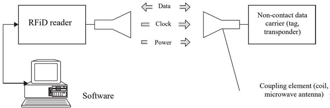
Fig. 2. The general structure of RFID system (source [1])
