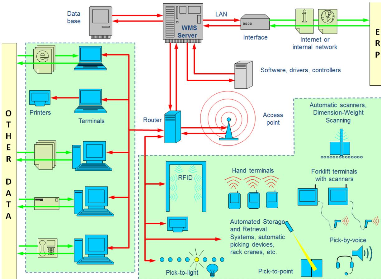
Fig. 1. The typical structure of WMS installation in logistics facility with supporting equipment.
