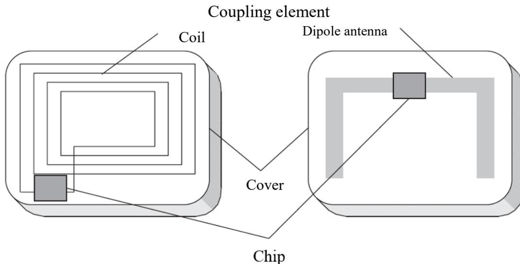
Fig. 3. The typical structure of RFID tag (source [1])
