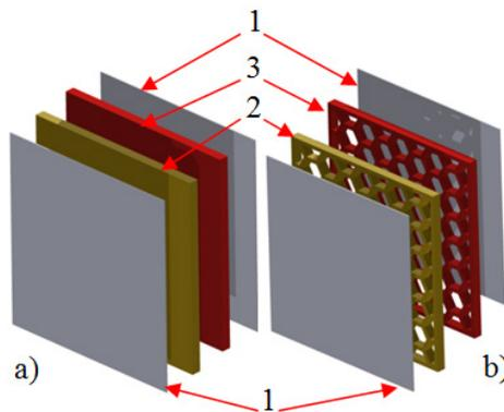
Fig. 1. Configuration of energy absorbing elastomer panels: a) without openwork structure, b) with openwork structure
