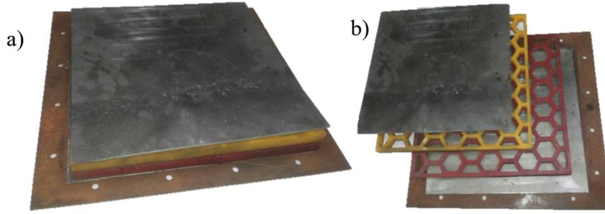
Fig. 6. Energy absorbing panels after experimental investigations: a) panel type A; b) panel type B
