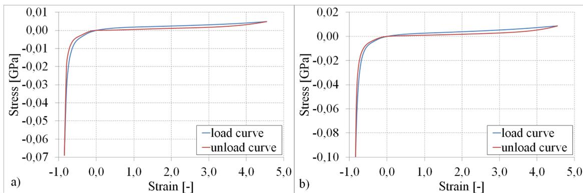
Fig. 5. Hysteresis loops of compression and tension for elastomeric materials: a) Asmaprene Q; b) Asmathane
