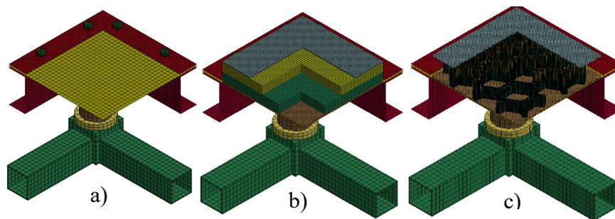
Fig. 4. Numerical models: a) test stand with protected plate, b) test stand with A type panel, c) test stand with B type panel
