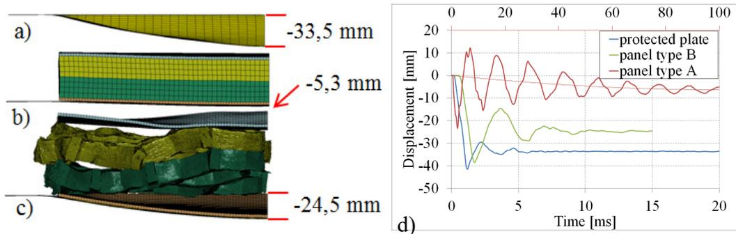
Fig. 7. Deflection of the protected plate based on the numerical analysis: a) protected plate; b) A type panel; c) B type panel; d) protected plate deflection waveforms in time
