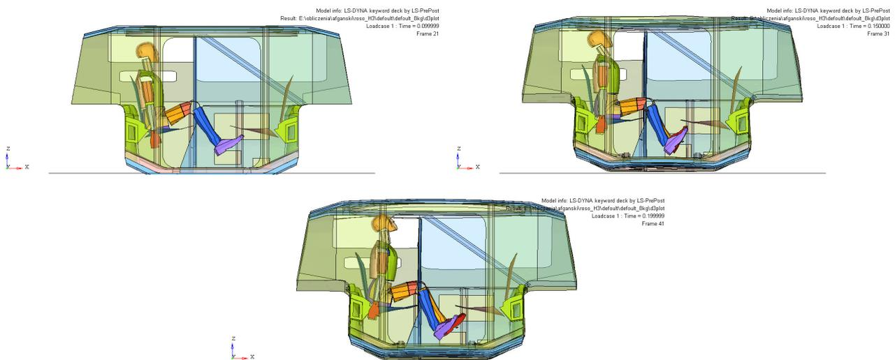
*Fig. 7. Hull deformation and dummy behaviour for subsequent moments of time during detonation of 8 kg of TNT*
