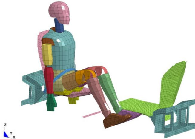
*Fig. 6. Dummy positioning*
