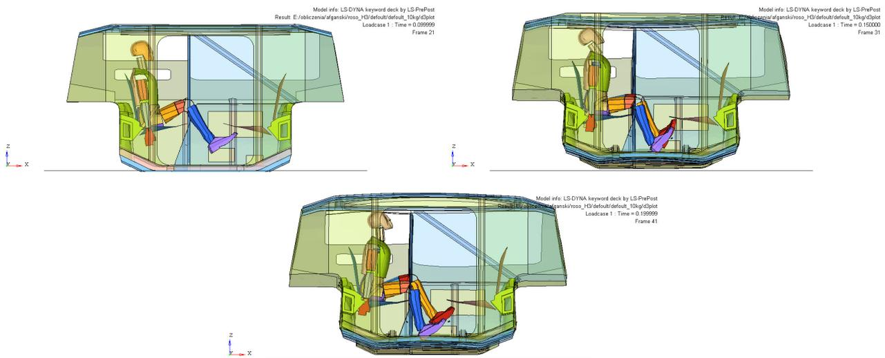
Fig. 10. Hull deformation and dummy behaviour for subsequent moments of time during detonation of 10 kg of TNT
