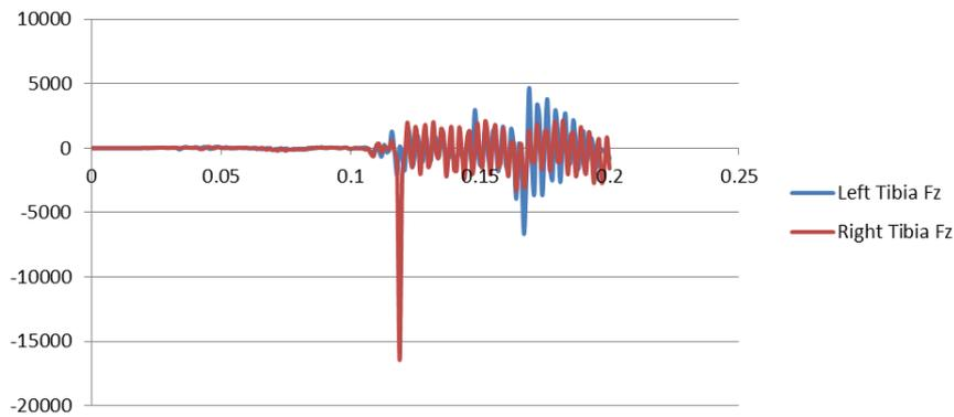
Fig. 9. Axial force in tibias [N] during detonation of 8 kg of TNT
