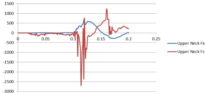
Fig. 11. Axial and transverse force in upper neck [N] during detonation of 10 kg of TNT
