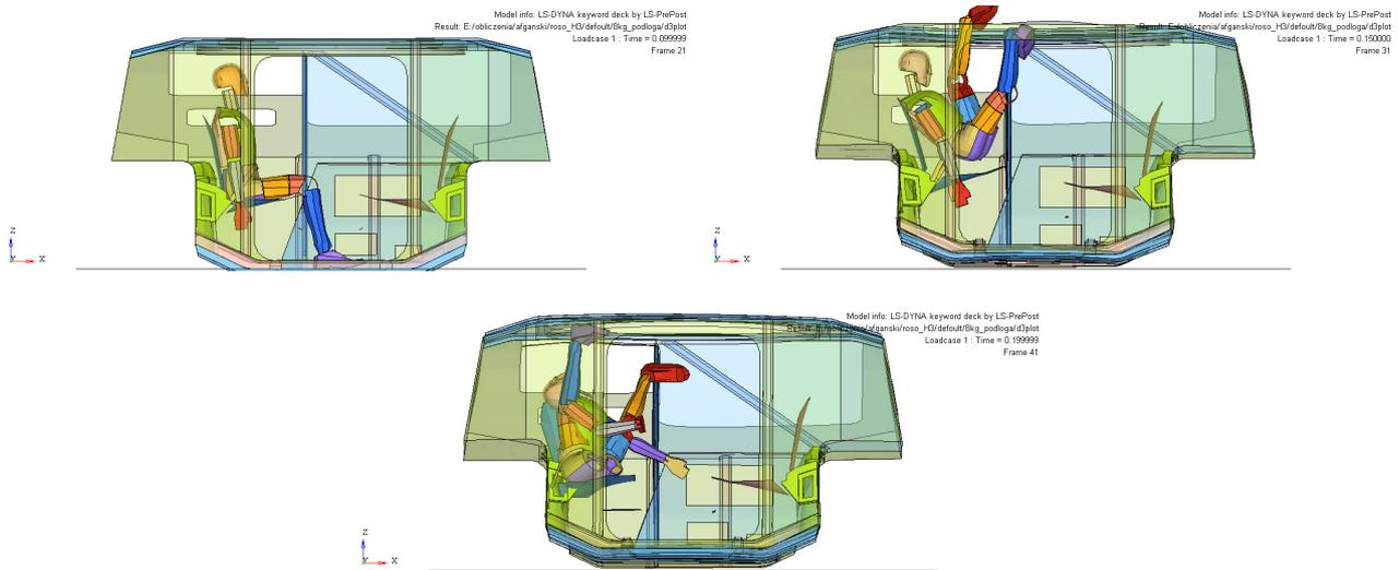
Fig. 13. Hull deformation and dummy behaviour for subsequent moments of time during detonation of 8 kg of TNT without footrest
