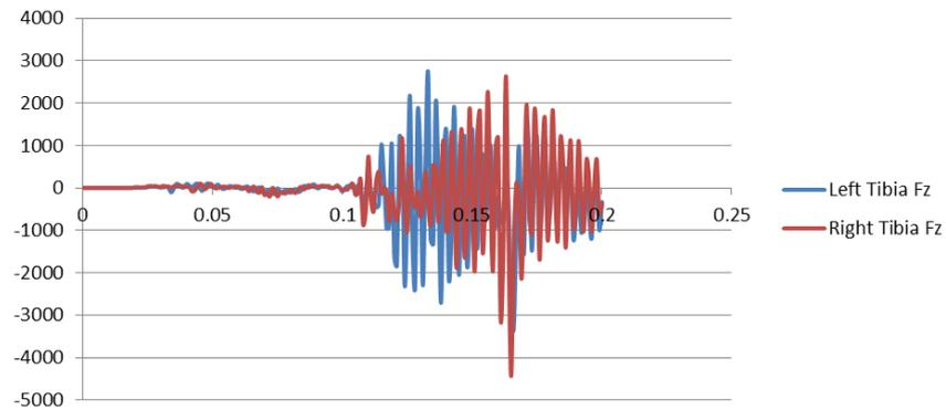
Fig. 12. Axial force in tibias [N] during detonation of 10 kg of TNT
