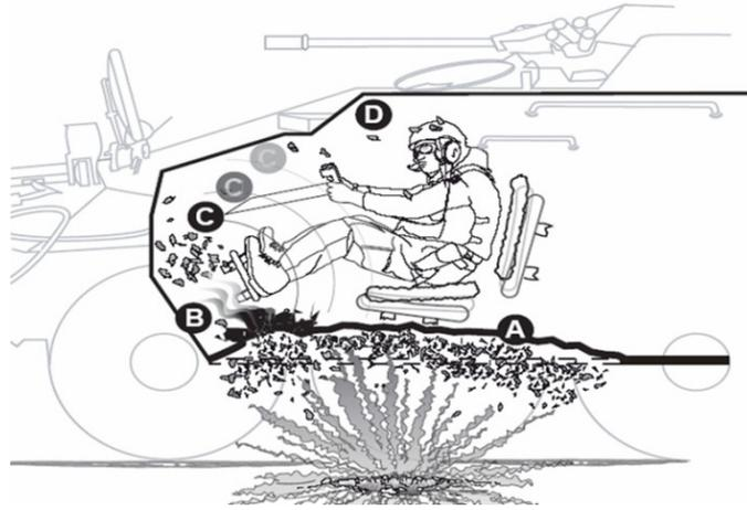
Fig. 1. Explosion effects under military vehicle: A – direct effects of explosion, B – toxic gas, C – overpressure due to detonation, D – fragments and projectiles [2]
