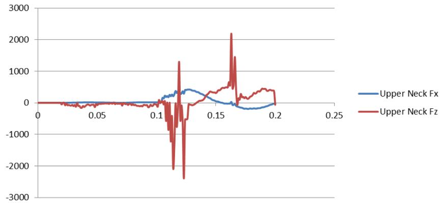
Fig. 8. Axial and transverse force in upper neck [N] during detonation of 8 kg of TNT
