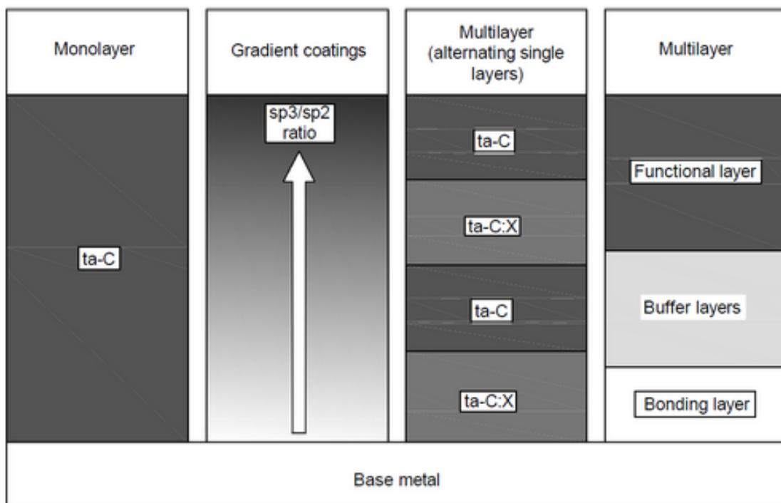
Fig. 5. Types of coatings in terms of layers number
