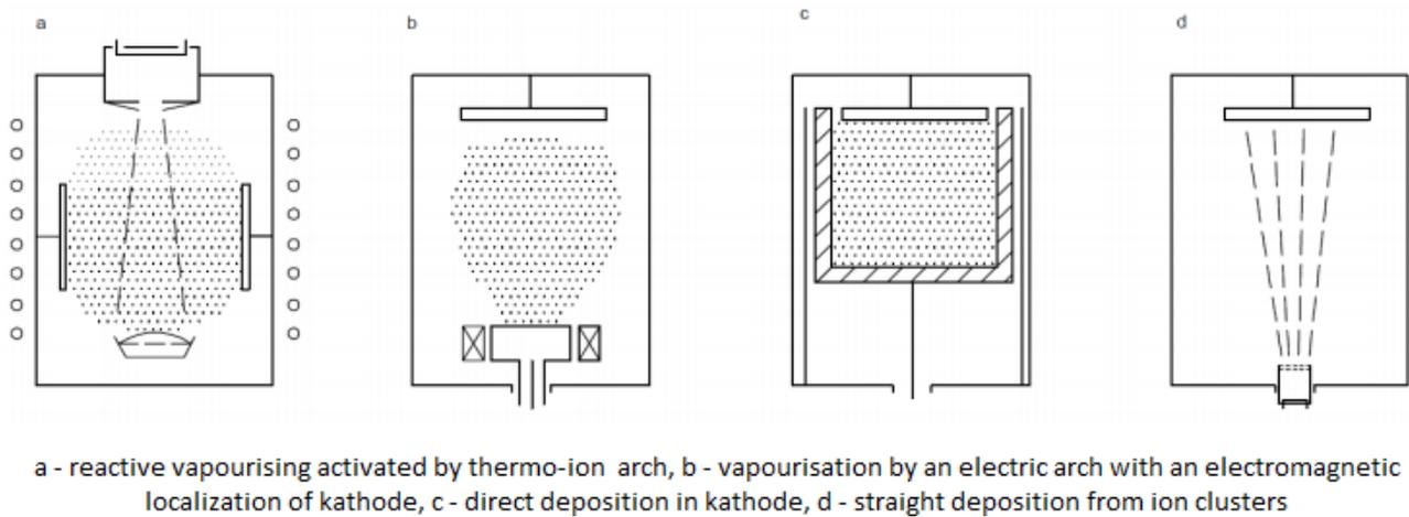
Fig. 4. Different PDV methods
