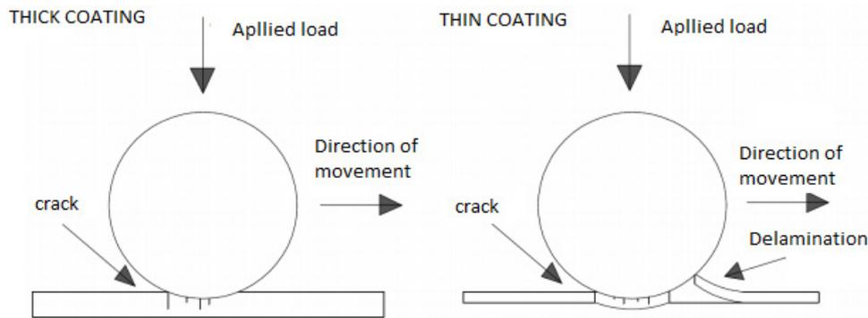
Fig. 1. Cracking of a coating in dependence of its thickness
