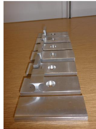
Fig. 4. View of combustion chamber models before testing
