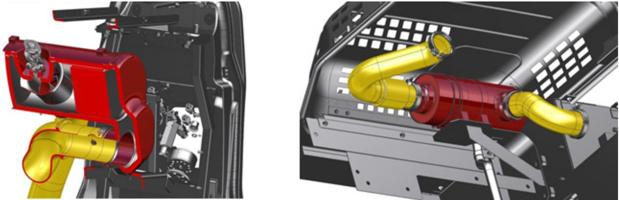
*Fig. 3. Inline concept of SCR system in HD application, left , right*
