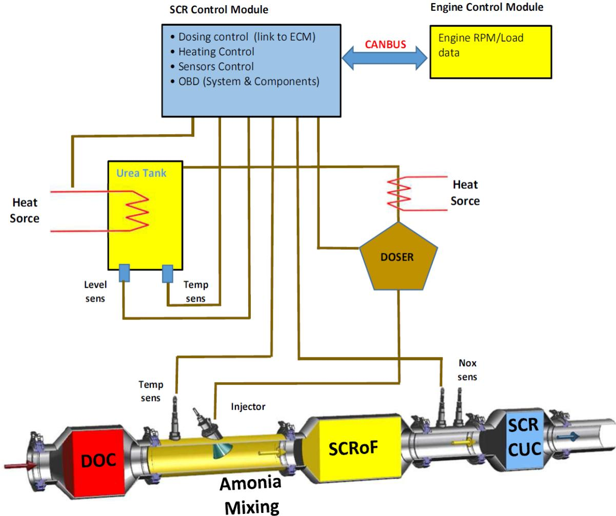
Fig. 1. Emission reduction system: DOC – oxidizing catalyst, SCR CUC – ammonia blockage filter
