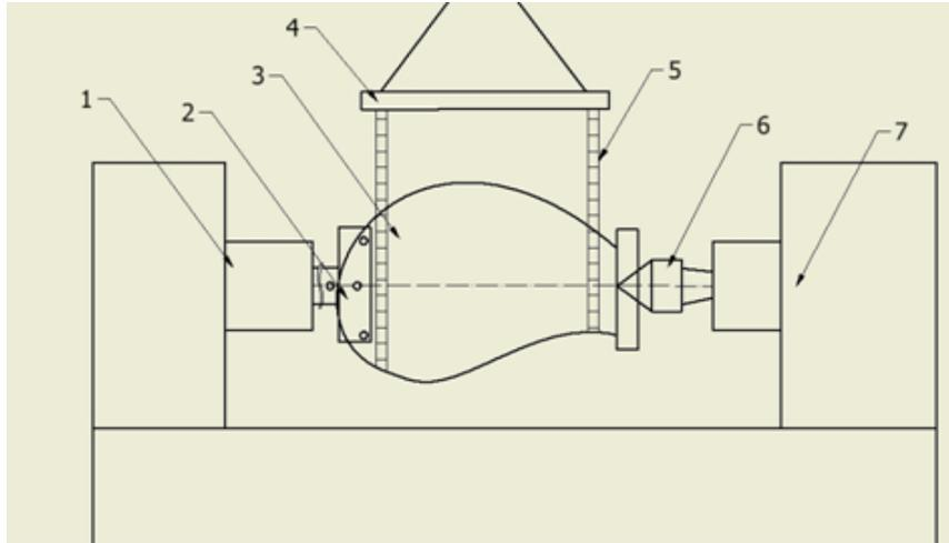
Fig. 2. Method of affixing propeller's wing in the lathe: 1. spindle, 2. handle, 3. workpiece, 4. mounting strip, 5. straps, 6. dead centre, 7. tailstock
