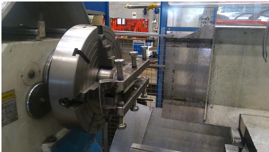
Fig. 4. The prototype handle for the processing of propellers wing thruster is mounted in the lathe
