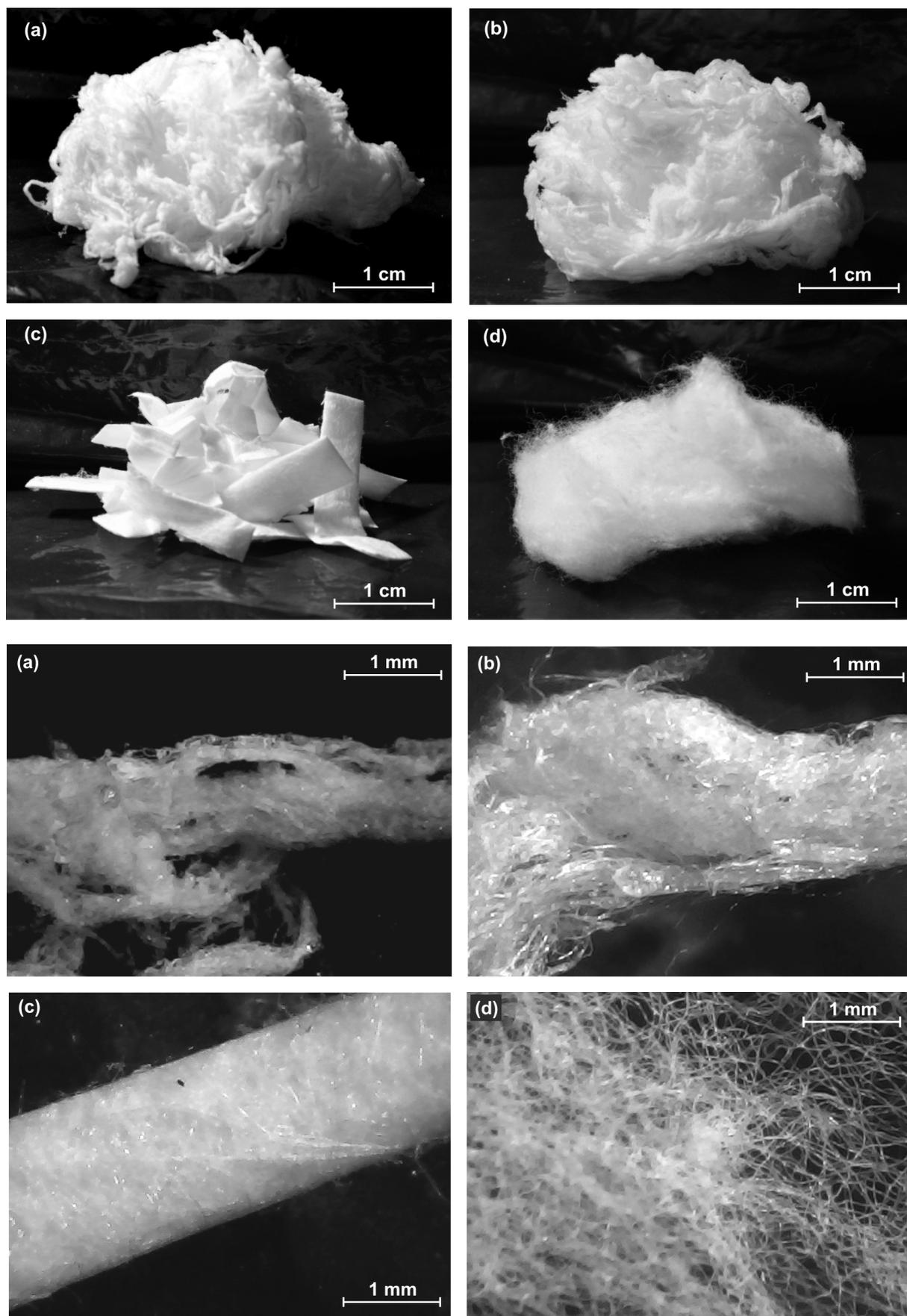
Fig. 1. Pictures of sorbents: (a) polypropylene wadding “winter”, (b) polypropylene wadding “summer”, (c) polypropylene nonwoven, (d) cotton wool
