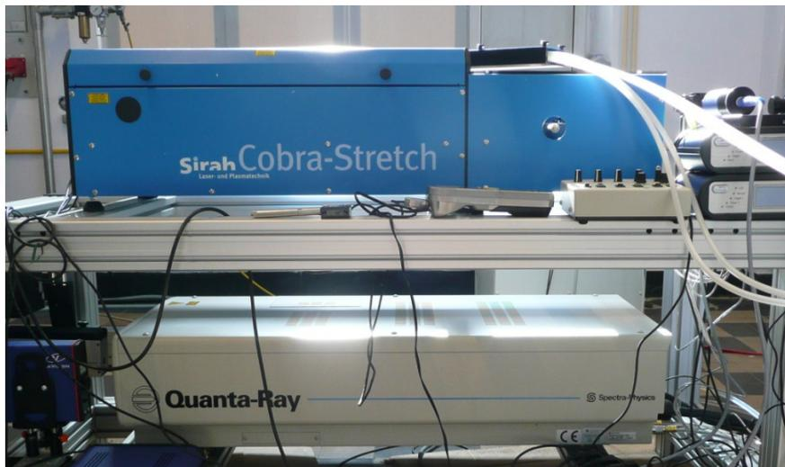
*Fig. 3. Sets of two lasers; Nd:YAG on bottom (pump laser), and dye on top*
