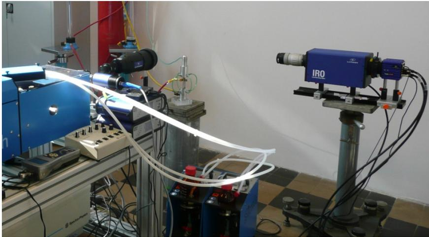
*Fig. 2. The system setup for LIF measurements*
