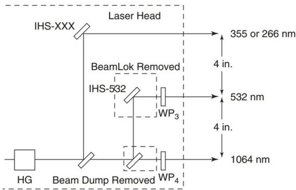
Fig. 4. The schematic optics providing functionality of generating 3 different wavelengths at the same time (1064 nm, 532 nm and 355 nm or 1064 nm, 532 nm and 266 nm); HG stands for harmonic generator and IHS for internal harmonic separator [4]
