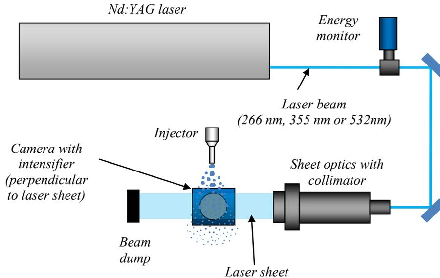
Fig. 11. Schematic setup of the system for LIF measurements
