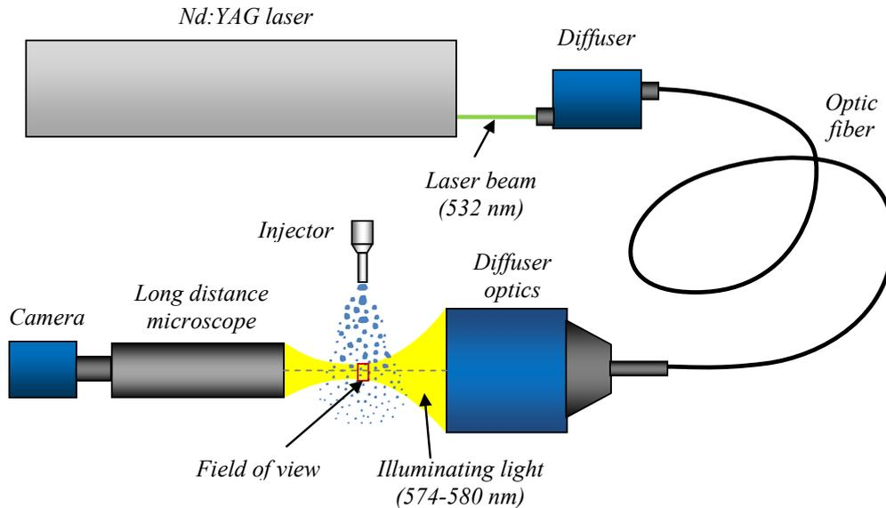
Fig. 7. Schematic setup of the system for shadowgraphy measurements
