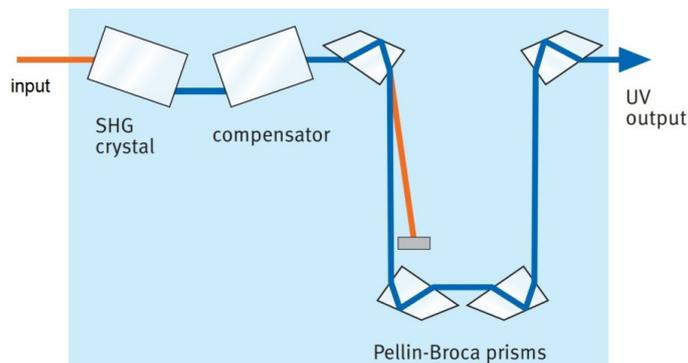
Fig. 6. The schematic optics of the SHG integrated with dye laser [6]
