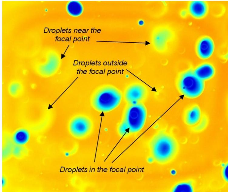
*Fig. 9. Example image of the droplets obtained by shadowgraph technique*
