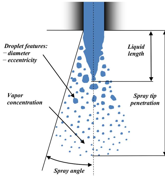
*Fig. 1. The main parameters used for spray characterization*
