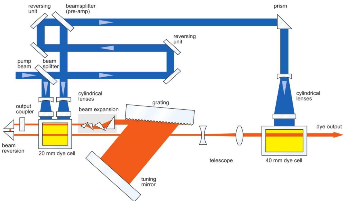
Fig. 5. The schematic optics of the dye laser; pump beam is the beam directed from Nd:YAG laser [5]
