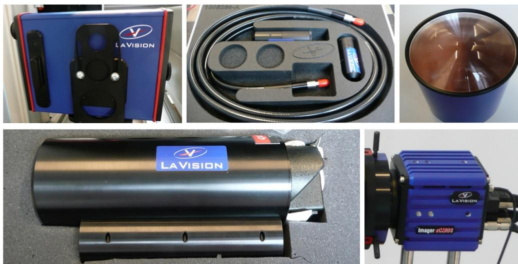
Fig. 8. Diffuser optics (on top) – diffuser, optic fibre and diffuser lens respectively from left, long distance microscope (bottom left) and sCMOS camera (bottom right)
