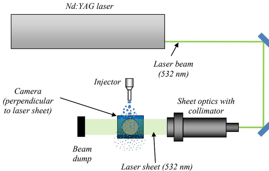
*Fig. 10. Schematic setup of the system for Mie scattering measurements*
