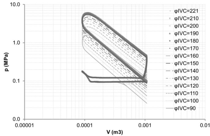
Fig. 2. Pressure vs. volume for different IVC
