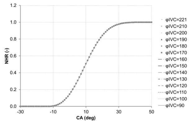
Fig. 8. HRR vs. CA for different IVC
