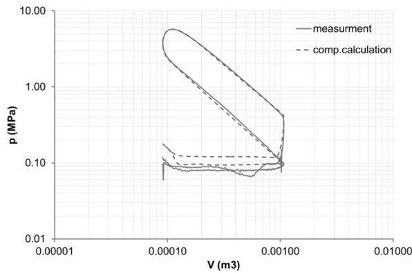
Fig. 1. Comparison between measured pressure trace and calculated pressure trace
