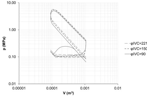
Fig. 11. Pressure-trace vs volume for three values of intake valve closure angle
