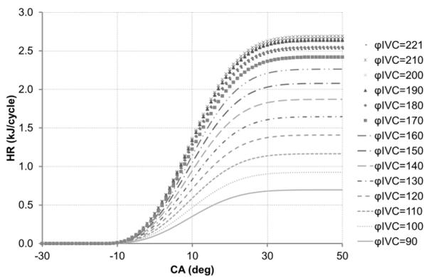
Fig. 7. HR vs. CA for different IVC
