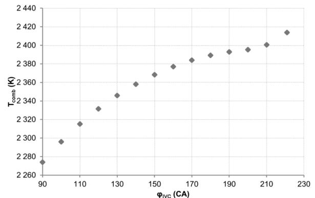
Fig. 6.  $T_{comb}$  vs. IVC
