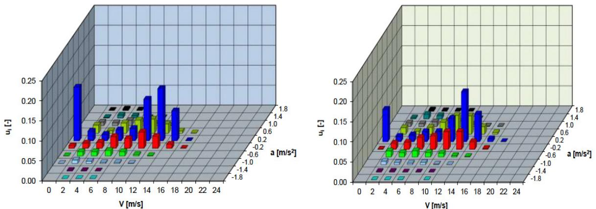
Fig. 5. Two-dimensional histograms of participation of the vehicle operation time during testing in coordinates of the vehicle speed - acceleration: ■ – vehicle I (CNG), ■ – vehicle II (diesel)
