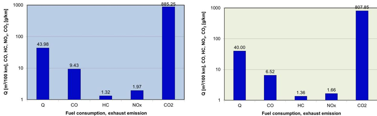
Fig. 11. Results of the road fuel consumption and the road emission of substances obtained during testing
