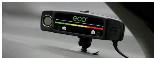
Fig. 8. The eco-panel of Sagasystem informing the driver in regards to the driving style: Green LEDs indicate ecological driving. Yellow LEDs indicate driving which strays away from the economical characteristics. Red LEDs indicate uneconomical driving
