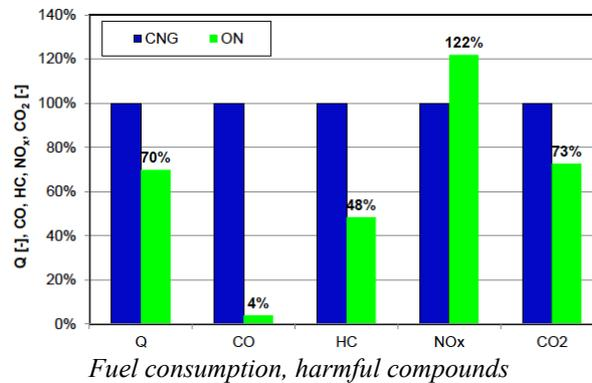
Fig. 7. Comparison of the road consumption of fuel and the road emission of pollutants, obtained during testing
