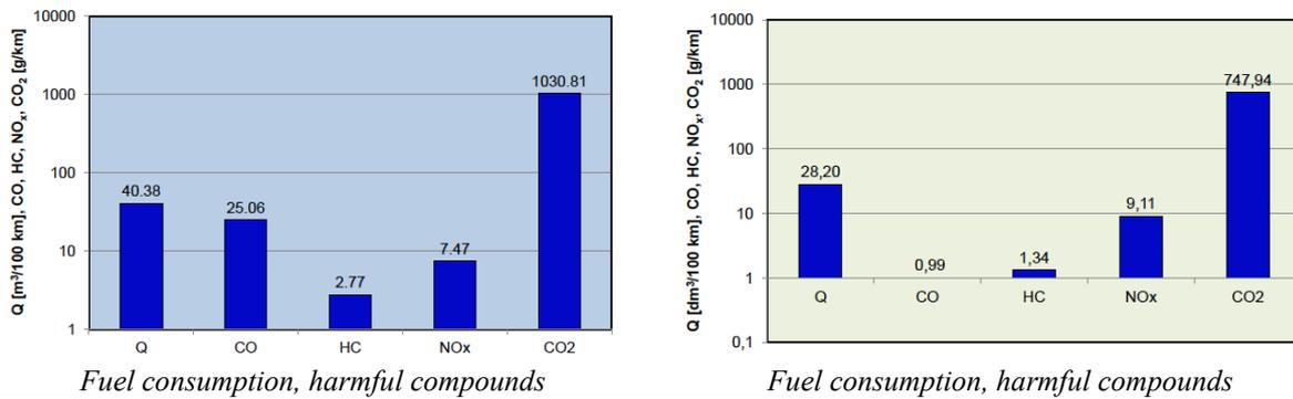
Fig. 6. The results of the mileage consumption of fuel and the road emission of pollutants, obtained during testing:
