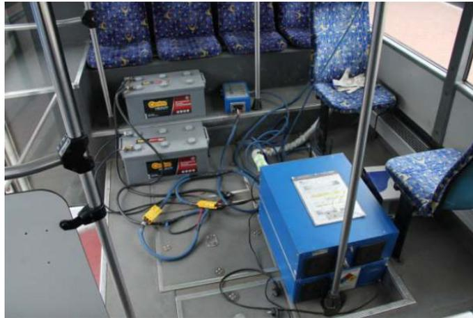
Fig. 3. One of two devices used to measurement exhaust pollutants under real conditions
